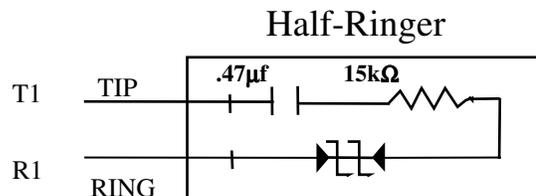
The half-ringer unit is essentially a two-connection device with terminals T1 and R1 connected to subscriber terminal wiring. The half-ringer is transparent to normal voice conversations and is not affected by the central office battery voltage. Once the half-ringer is activated, it will function as termination by permitting current to flow through it, but only when an alternating voltage of nominal 5.4 volts is present at the termination.
