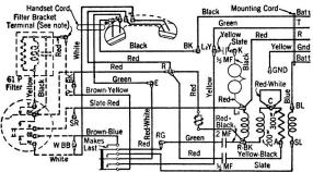
Note: If filter is not provided connect brown yellow lead from switch contacts to Y of dial instead of to filter terminal bracket Terminals Y-BK,SR and W-BB are on the manual set apparatus blank.
