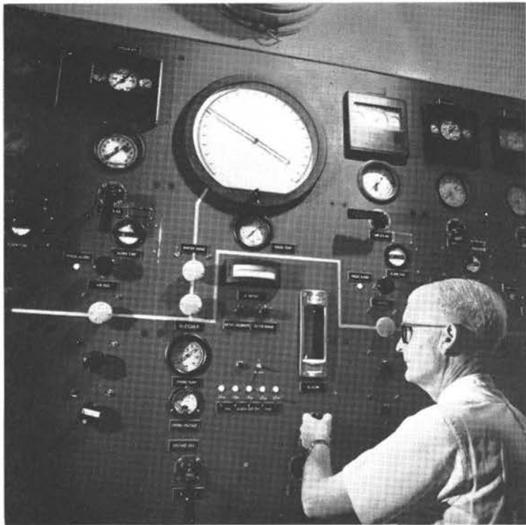
During cable tests, tension and pressure are varied to simulate actual laying process. Starting tension applied in tests is 7900 pounds, while terminal pressure is 5000 psi. P. W. Rounds operates control panel for the sixteen artificial oceans.
