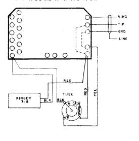
CONNECTIONS FOR A - TIP STATION FOR A - RING STATION CONNECT TUBE AND RINGER LEADS AS SHOWN BUT CONNECT RING OF LINE TO L-2 AND TIP OF LINE TO L-1.
