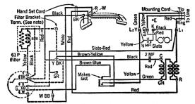
Note: If filter is not provided connect brown-yellow lead from the switch contacts to Y of dial instead of to filter bracket terminal. Terminals Y-BK,SR and W-BB are on the manual set apparatus blank.
