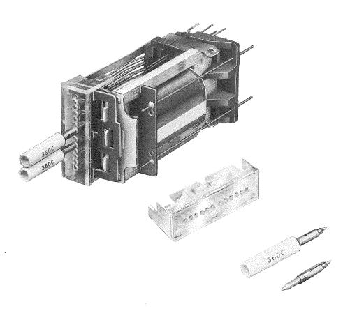
Fig. VIII-1 - Method of Connecting to Fixed Contacts
