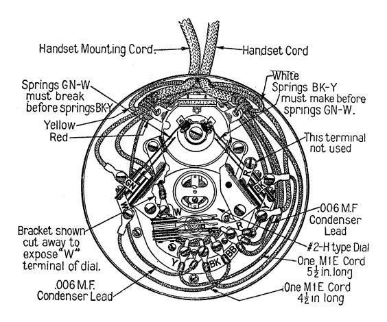
Cord tips are placed with flat side down (where joint is shown dark) and up (where shown white), to prevent crosses or grounds.
