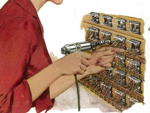
With one quick zip, this "gun"—developed jointly by Bell Telephone Laboratories and Western Electric —wraps wires on telephone equipment so tightly
