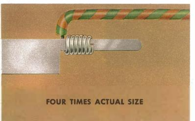
At Western Electric, where we make a billion wired connections a year, this new method speeds production and cuts costs. Such savings help to hold down the cost of telephone equipment—and in turn help hold down the price of Bell telephone service.
