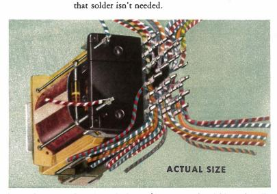
**Now, for example,** 36 terminals can be connected quickly and easily even in the small space provided in the relay above. That leads to savings in our job as manufacturing unit of the Bell System.
