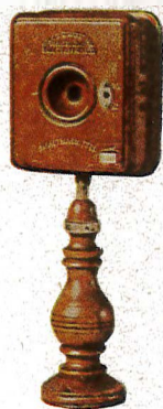
1880 Blake. Invented by Francis Blake, Jr., this new set was able to transmit the voice with greatly increased clarity.
