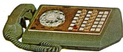
1958 Call Director® Telephone. Multi-purpose business phone, equipped with up to 30 pushbuttons for handling calls.
