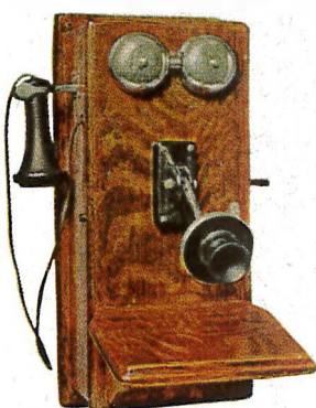
1907 Magneto Wall Set. A more modern version of the phone with a built-in generator for signalling the operator.
