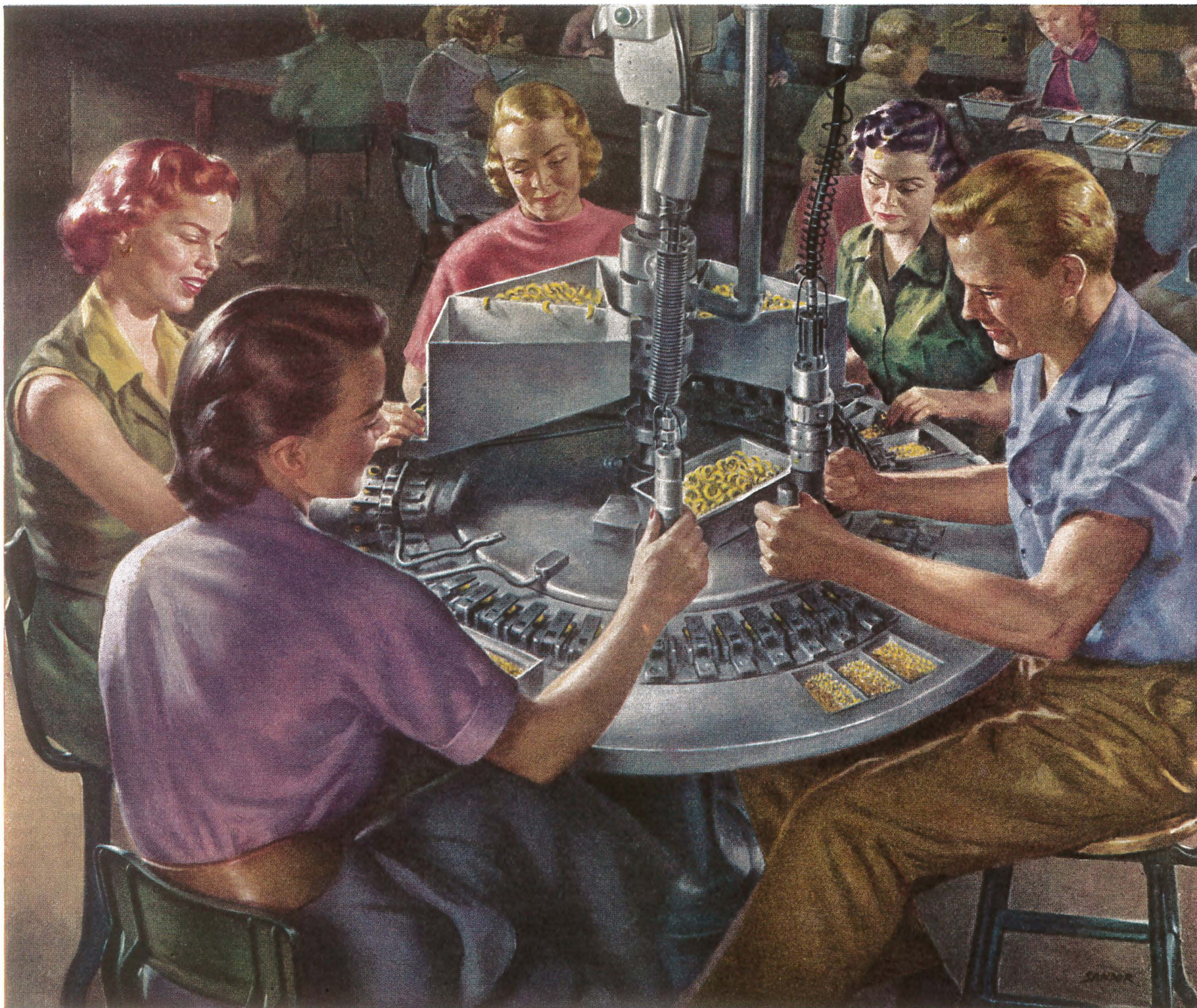
A Western Electric production team assembling devices which control the speed of Bell telephone dials.
