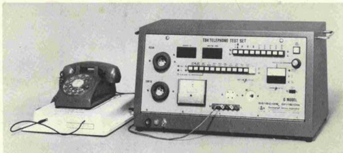
TYPICAL TEST SETUP USING THE T84 G MODEL TELEPHONE TEST SET AND T6 BREAKDOWN BASE
