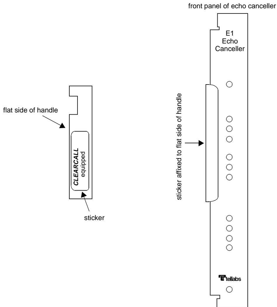
**Figure 5-1** CLEARCALL sticker placement on front panel handle of echo canceller
