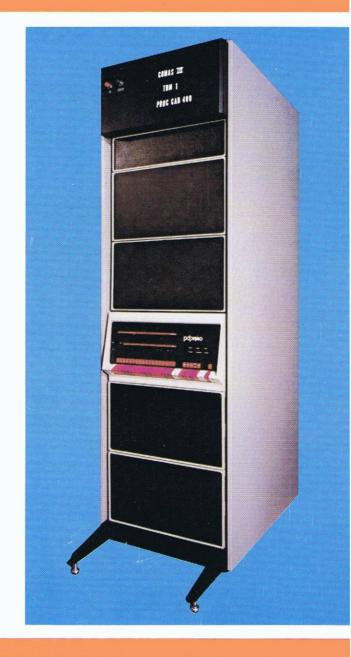
COMAS III is an on-site, stand-alone minicomputer system. It collects trouble data from existing trouble recorder circuits. Performs analysis. Formats the data. And shoots out hard-copy exception reports pinpointing defective equipment or combinations of equipment.
