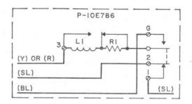
Note 1: The 174CT, GT coin collectors are equipped with P-10E786 coin relays wired as shown above.
