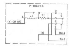
Note 1: 176CT, GT coin collectors are equipped with P-10E786 coin relays wired as shown above.
