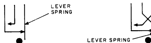
Fig. B—Special Make-Before-Break Contact Springs
