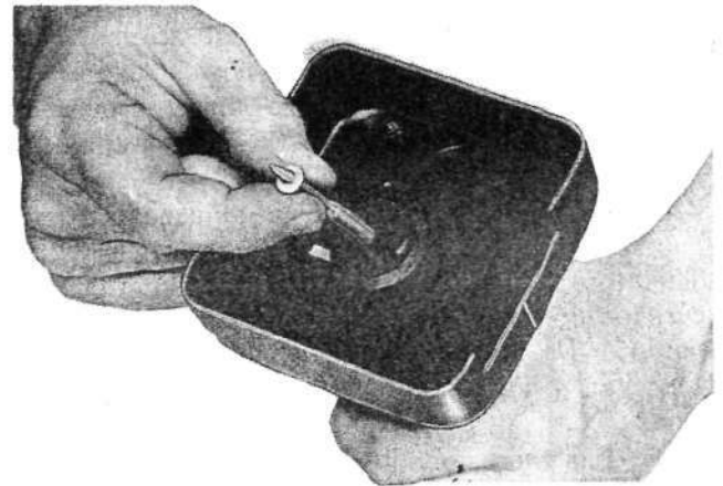
STEP 1 PLACE MASONRY FASTENER IN BUSHING FIRST.
