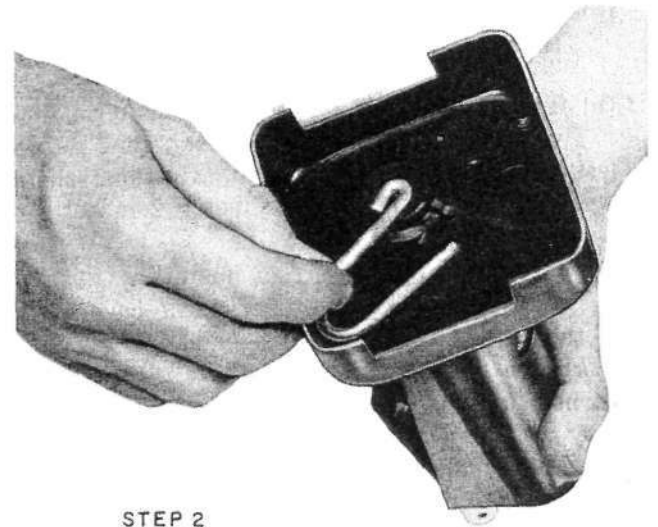
STEP 2 BE SURE WIRE LOOP IS HELD BY SPRING LOADED CATCH.
