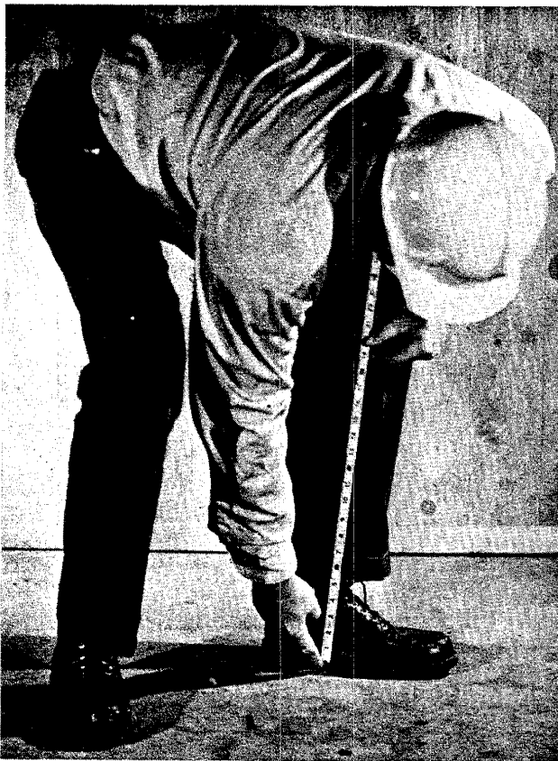
Fig. 8 — Measuring for Climber Length
