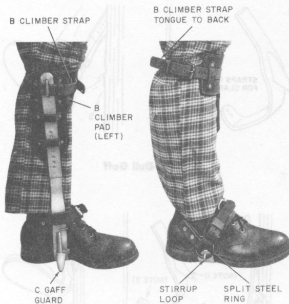
Fig. 9—Climber Strapped to Leg
