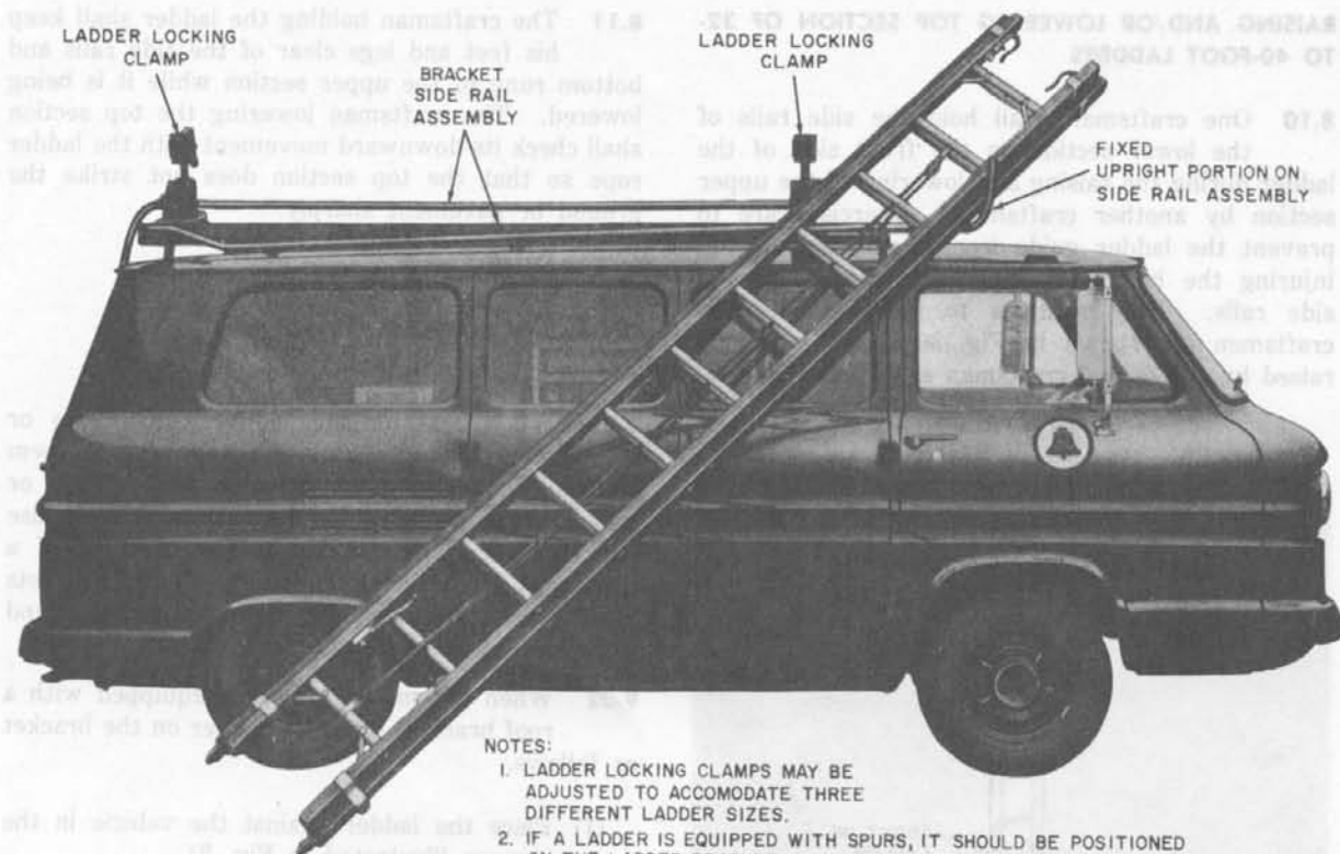
Fig. 31—Placing Ladder on Roof-Mounted Ladder Bracket
