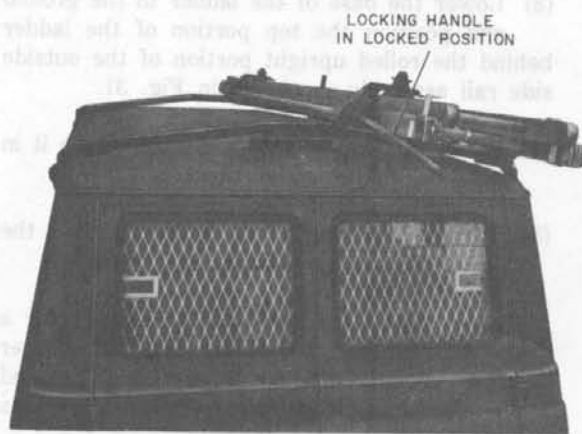
Fig. 32—Ladder Locked in Position on Roof-Mounted Ladder Bracket
