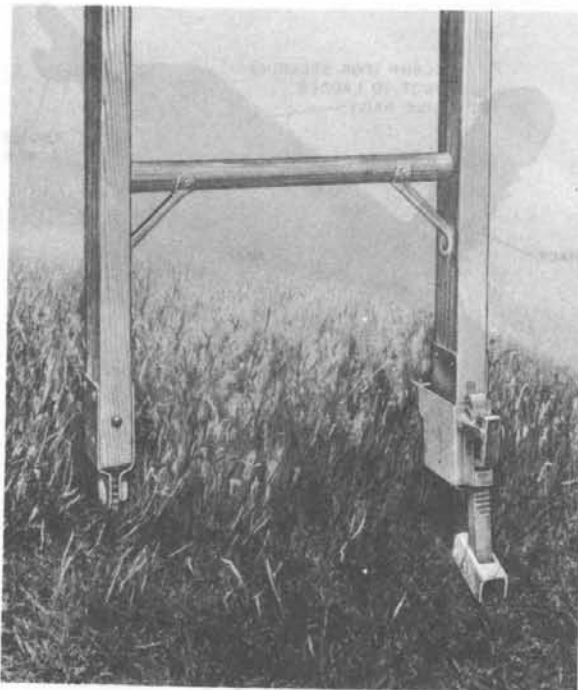
Fig. 7—B Ladder Foot Installed
