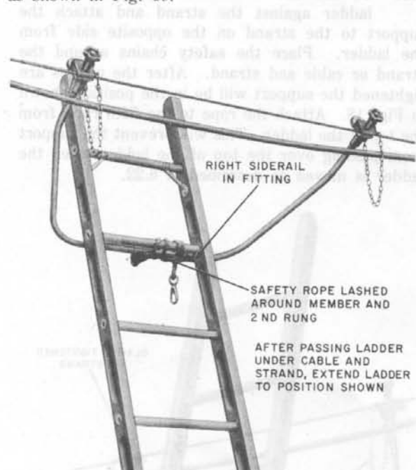
Fig. 19—C Ladder Support in Use
