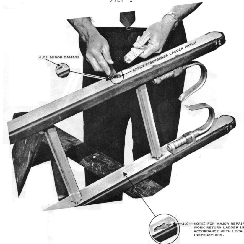
REPAIRING GOUGES IN SIDE RAILS FIGURE 5A
