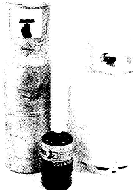
Fig. B: Propane and MAPP gas tanks
