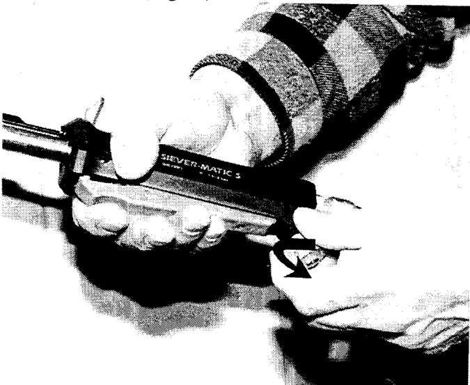
Fig. P: Open gas valve on handle
