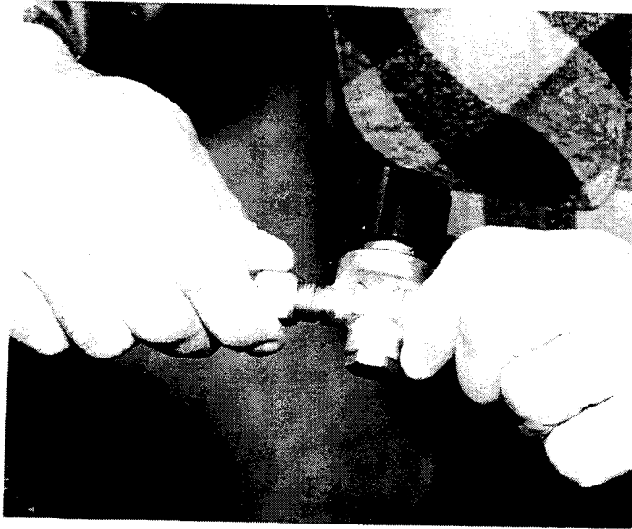
Fig. I: Attach hose to regulator
