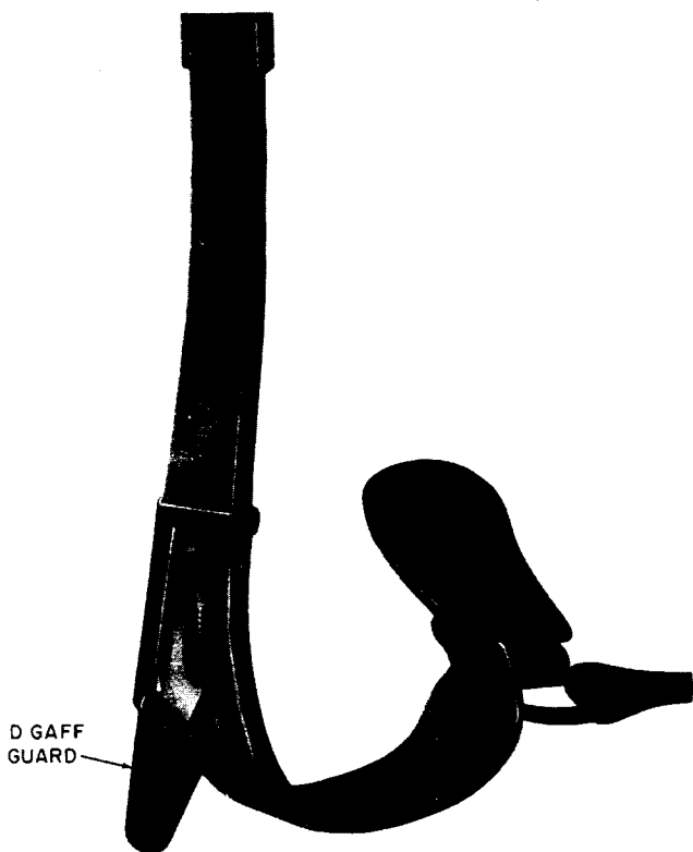
Fig. 8—D Gaff Guard Installed
