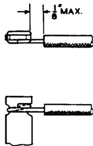
Fig. 14 — Single- or Double-Notched Terminals
