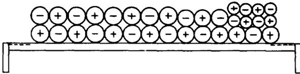
**Fig. 21 — Pairing of Talking Conductors on Cable Rack—Typical Section (See 2.03)**
