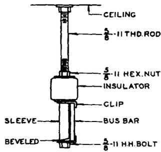
Fig. 6 - Bus-Bar Support from Ceiling - One Bus Bar
