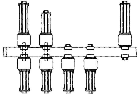
Fig. 9 - Typical Bus-Bar Support Arrangements
