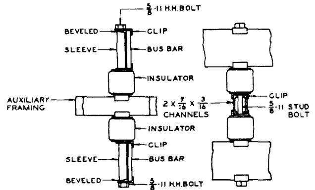
**Fig. 4 - Bus-Bar Support - Double-level Bus Bar**
