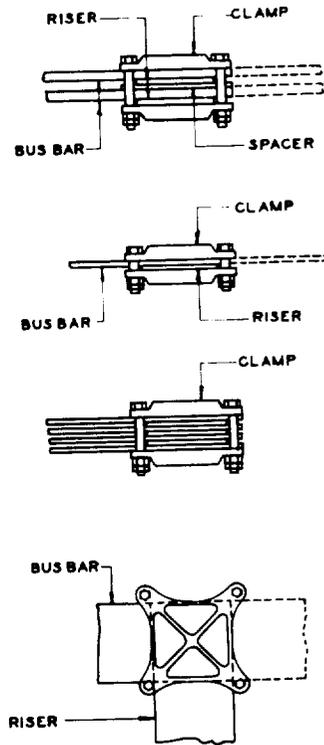
Fig. 12 — Bus-Bar Riser Joints
