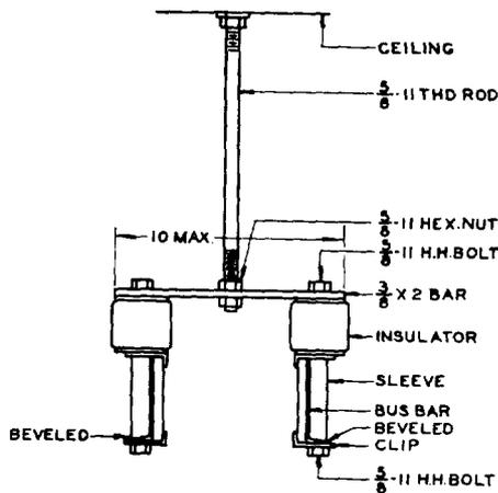
Fig. 8 - Bus-Bar Support from Ceiling - Same Level
