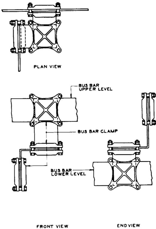
Fig. 11 — Typical Bus-Bar Connections with Intermediate Clamp
