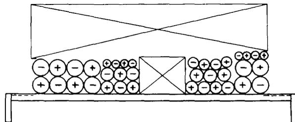
Fig. 20 - Power and Switchboard Cable on Cable Rack - Typical Section
