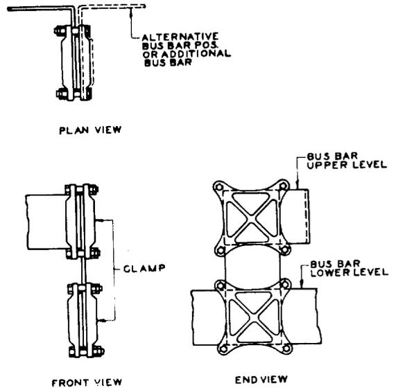
Fig. 13 — Typical Bus-Bar Connections
