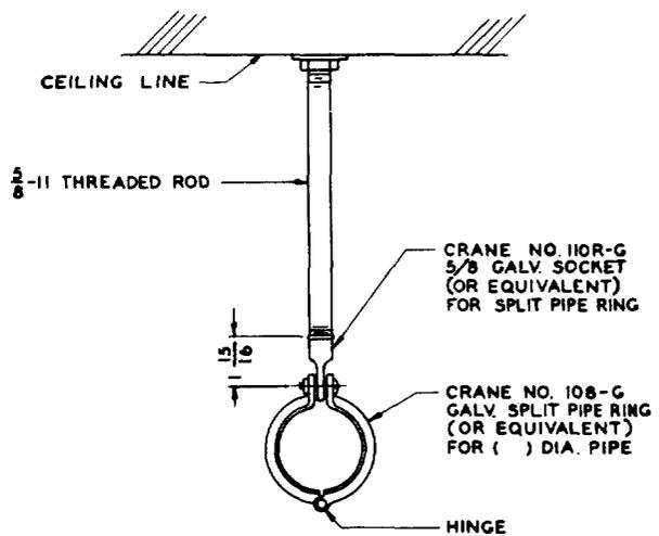
Fig. 24 — Conduit Support for Single Conduit Where Auxiliary Framing is Not Used
