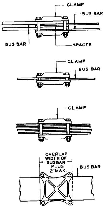
Fig. 10 — Bus-Bar Splice Joints
