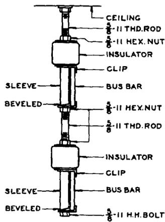
Fig. 7 - Bus-Bar Support from Ceiling - Two Levels
