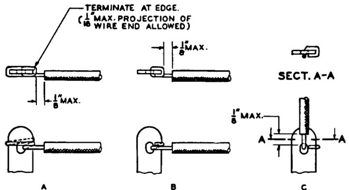
Fig. 15 — Drilled or Punched Terminals
