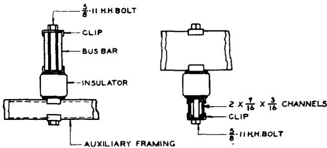
**Fig. 2 - Bus-Bar Support - Two Bus Bars**
