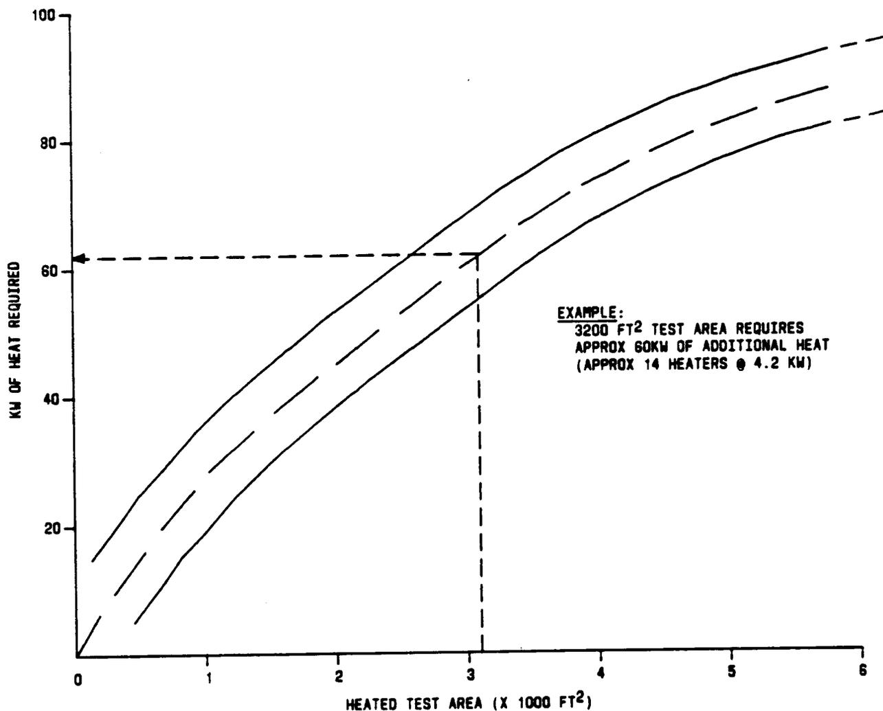
Figure 3. Heat Required for Test Area
