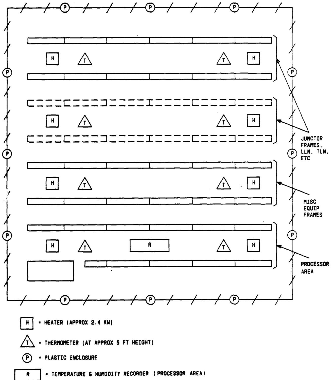
Figure 1. SPCS Heat Test - Typical Office Layout
