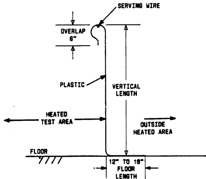
Figure 5. Establishing Panel Lengths
