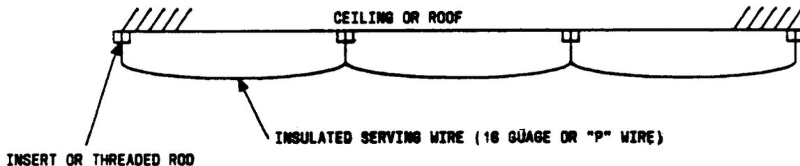
Figure 4. Serving Wire Installation
