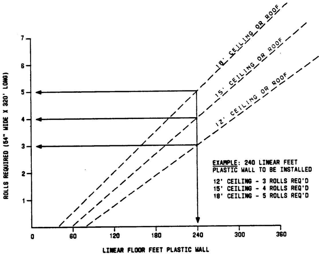
Figure 2. Amount of Plastic Sheeting Required for Heat Test Enclosure
