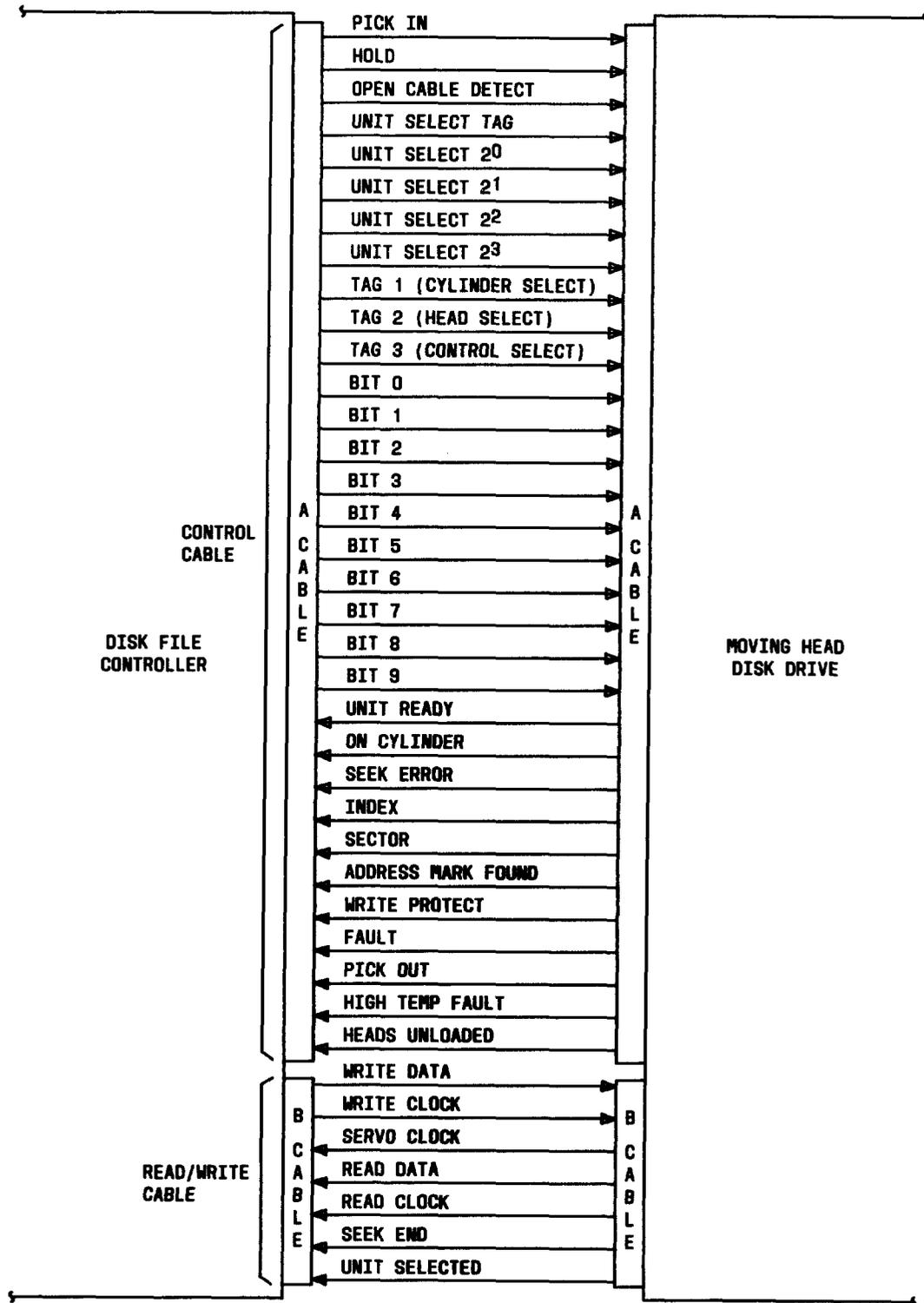
Fig. 8—Control and Read/Write Cables
