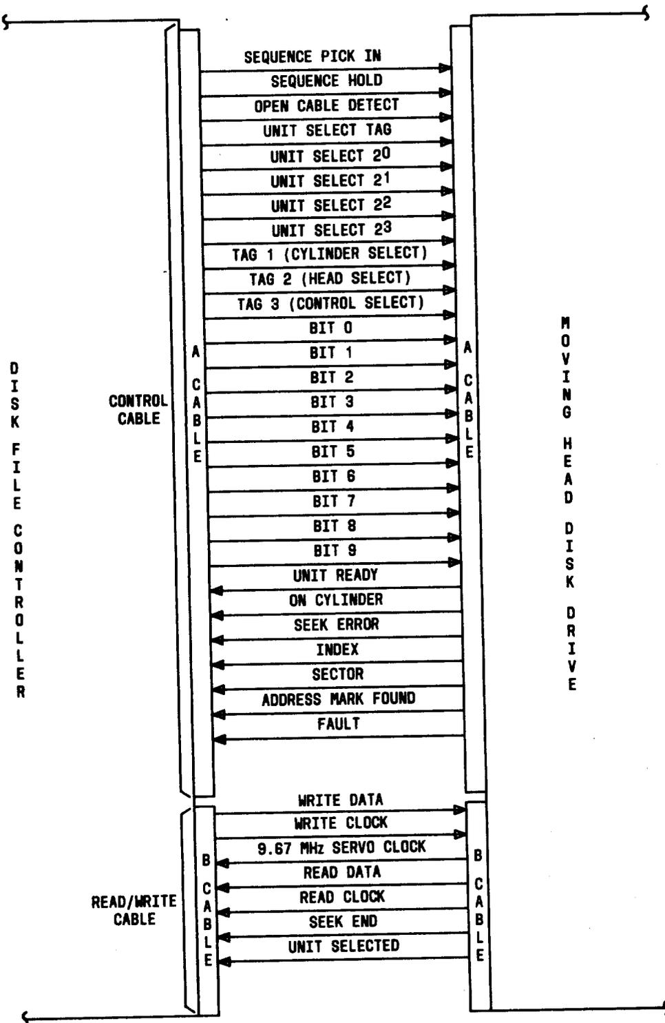
Fig. 7—Control and Read/Write Cables
