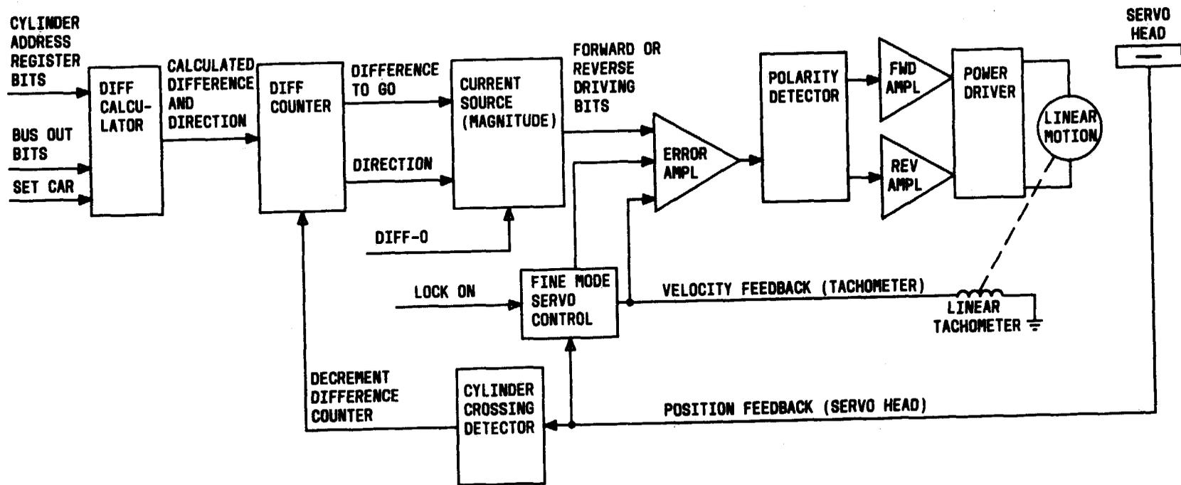
Fig. 10—Basic Servo Block Diagram
