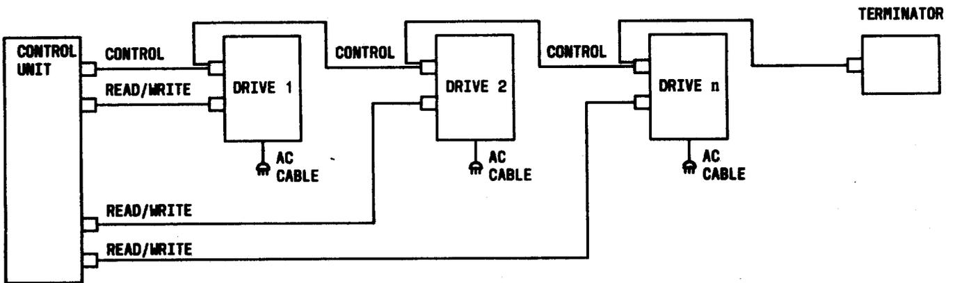
Fig. 8—System Daisy-Chain Configuration
