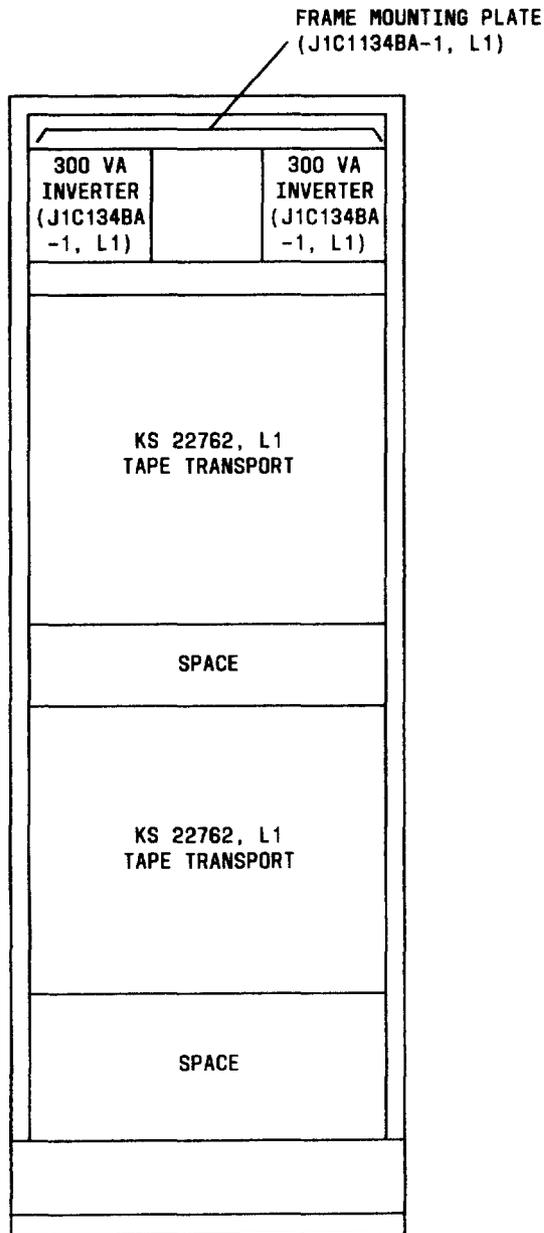
Fig. 2—Tape Transport Frame
