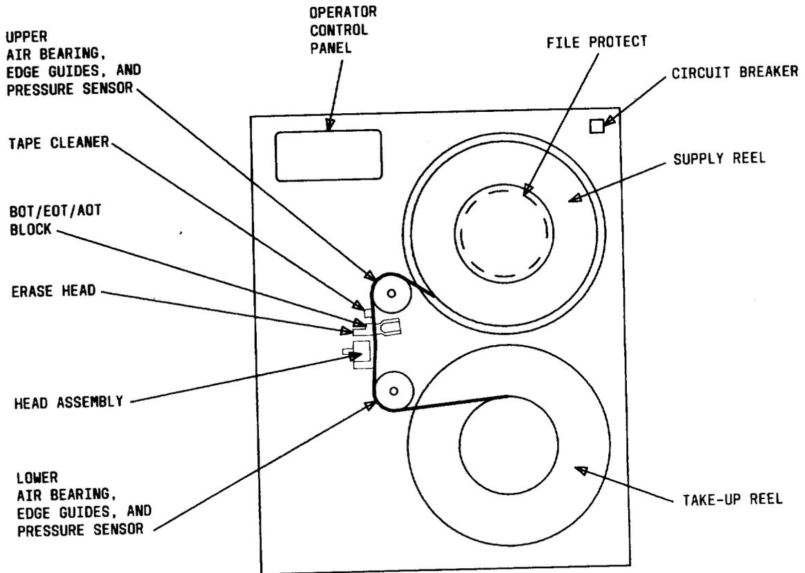
Fig. 5—Tape Deck (Front View)
