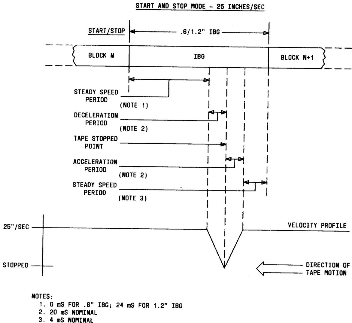
**Fig. 16—Start/Stop Mode Tape Motion Control**
