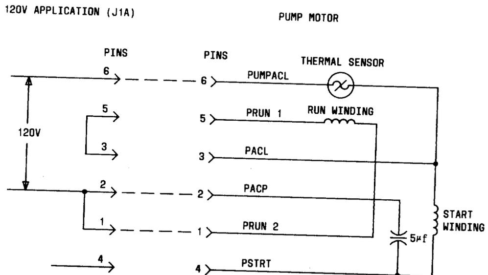
Fig. 14—Pump Motor Wiring Diagram
