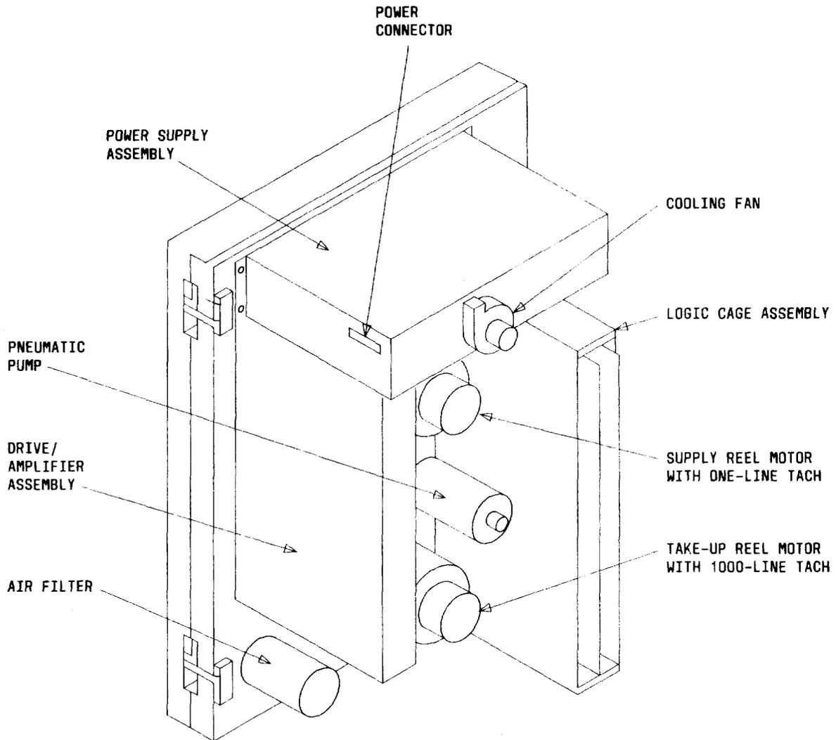
Fig. 6—Tape Deck (Rear View)
