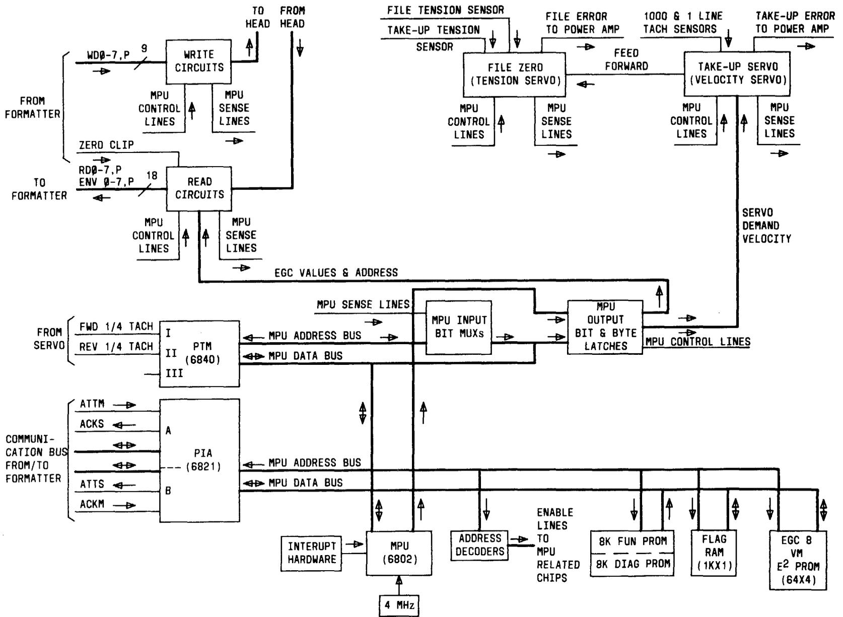
Fig. 9—Read/Write Servo Block Diagram
