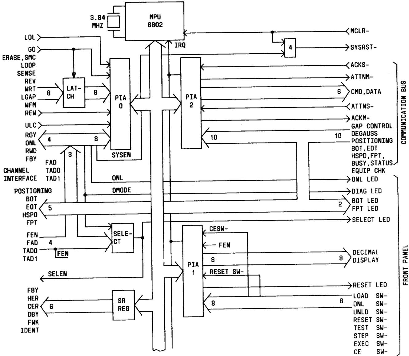
Fig. 8—Formatter/Control Block Diagram (Sheet 1 of 2)
