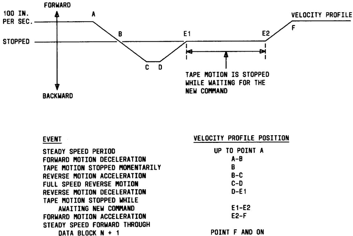
Fig. 21—Transport Velocity Diagram (Receiving Command Following Repositioning Cycle)
