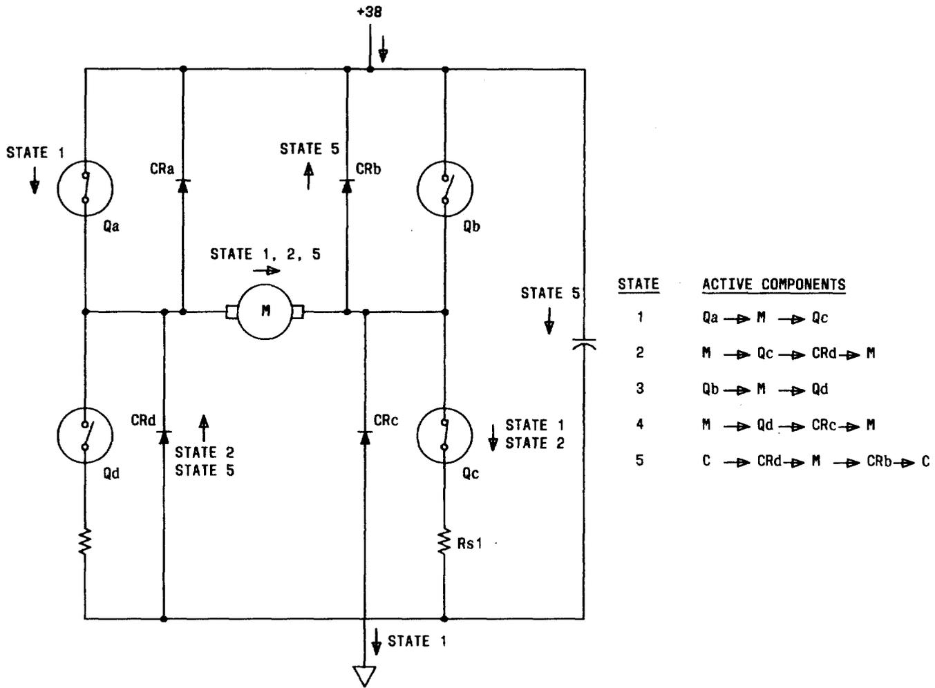
Fig. 12—Bridge Circuit
