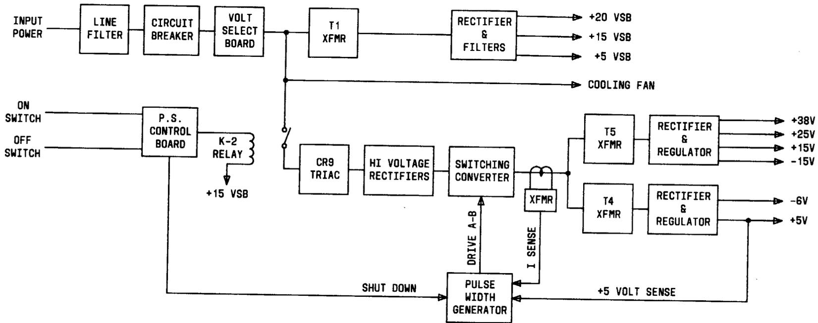
Fig. 10—Power Supply Block Diagram
