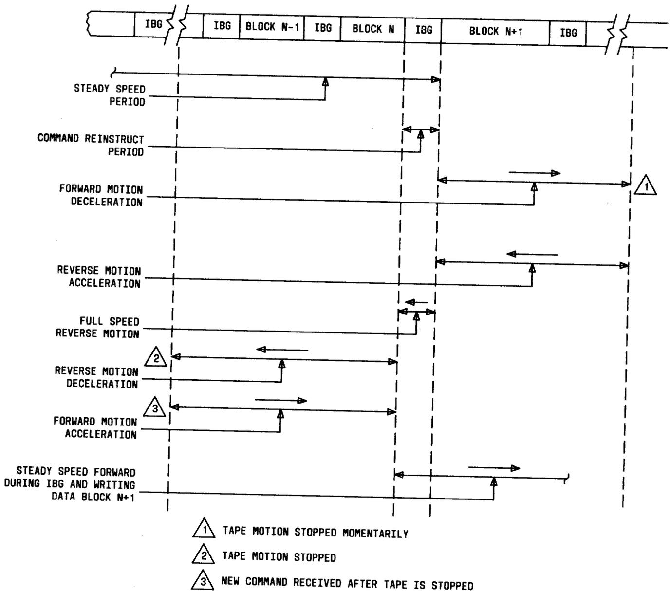
Fig. 22—Tape Motion Control (Receiving Command Following Repositioning Cycle)
