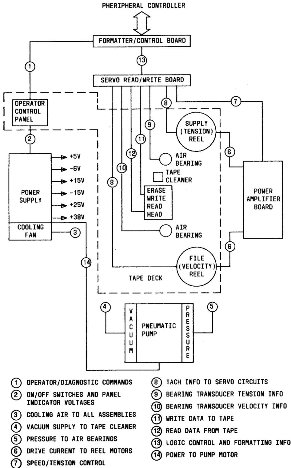
Fig. 7—Tape Unit Functional Block Diagram
