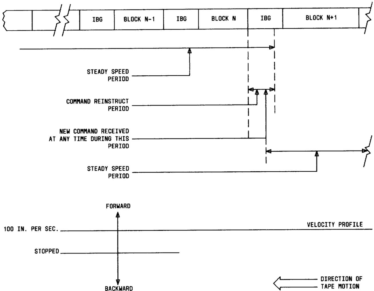
Fig. 18—Tape Motion Control (Nonstop)
