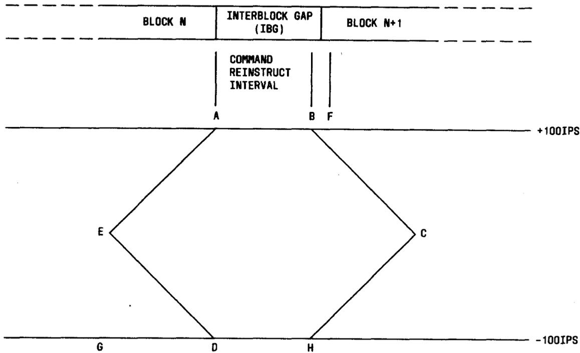
Fig. 17—Streaming Mode Velocity Diagram
