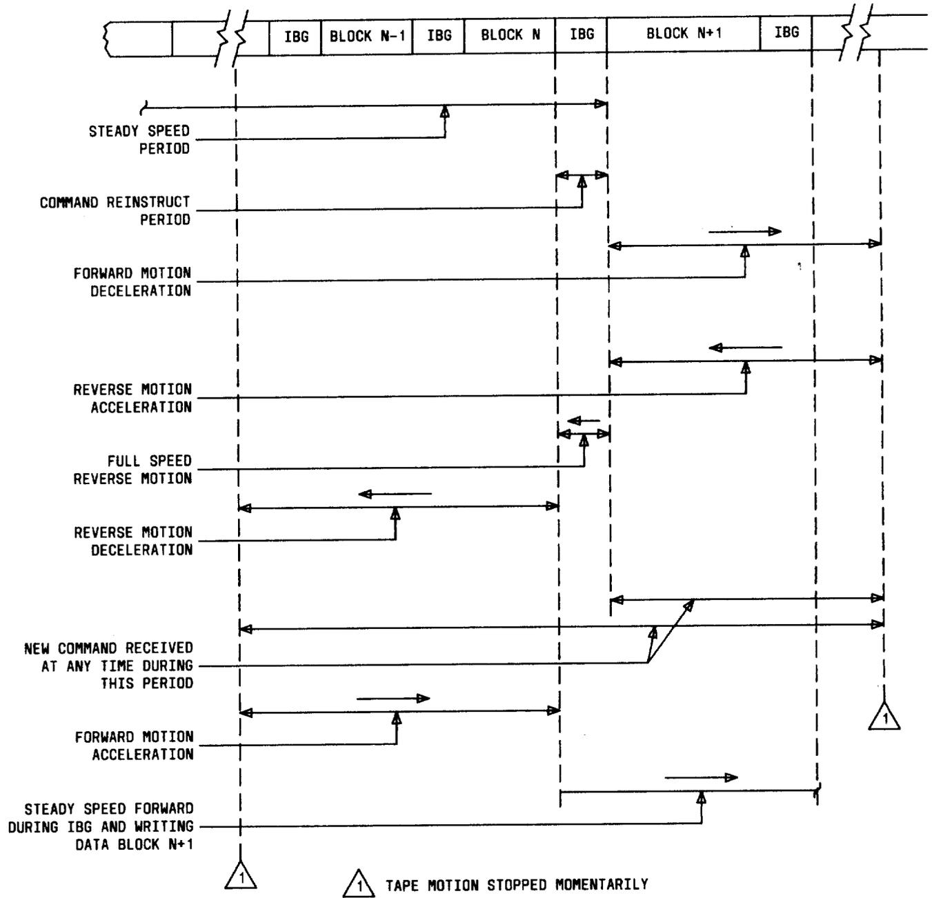
Fig. 20—Streaming Mode Tape Motion Control (Momentary Stop)
