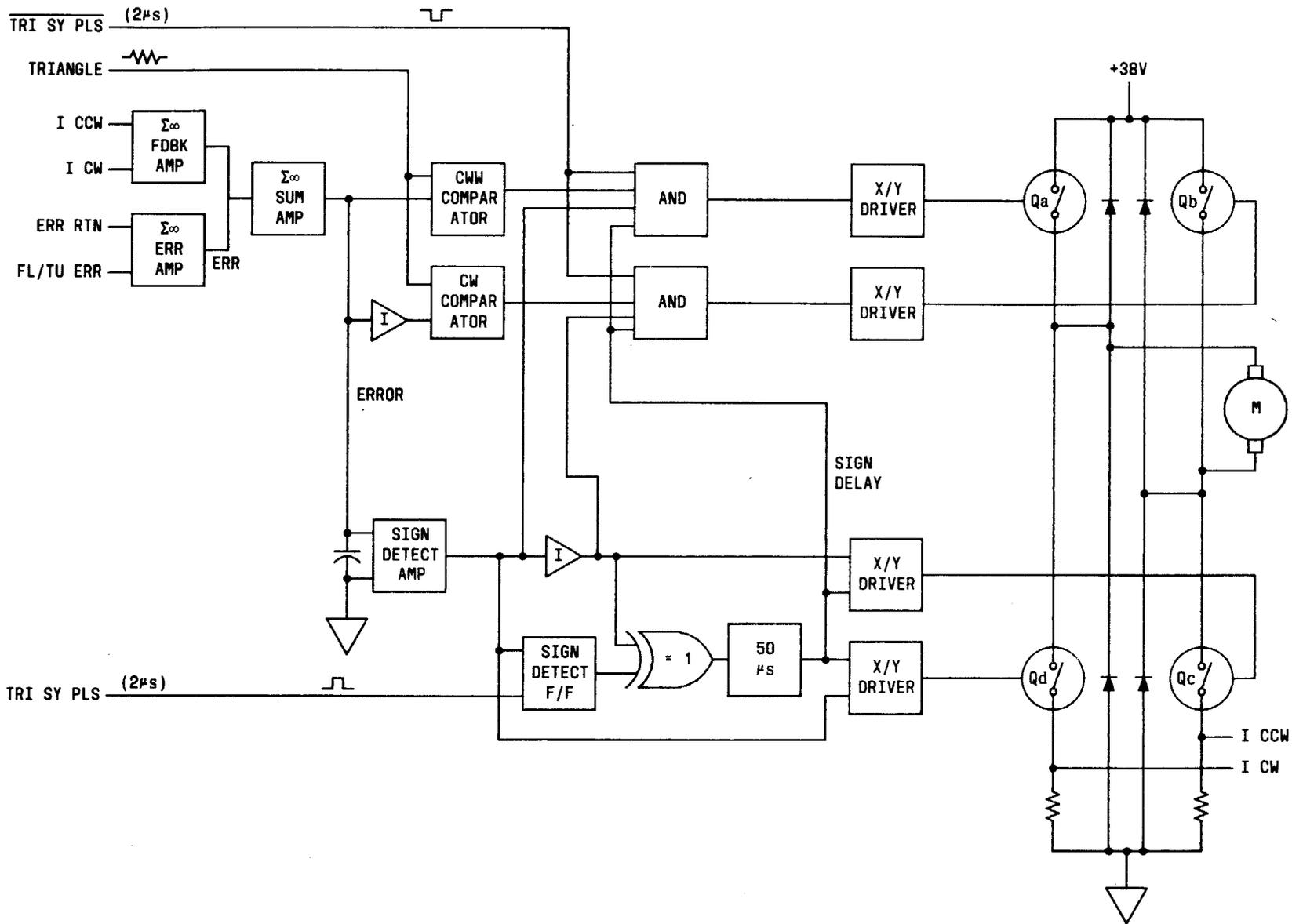
Fig. 11—Power Amplifier Block Diagram
