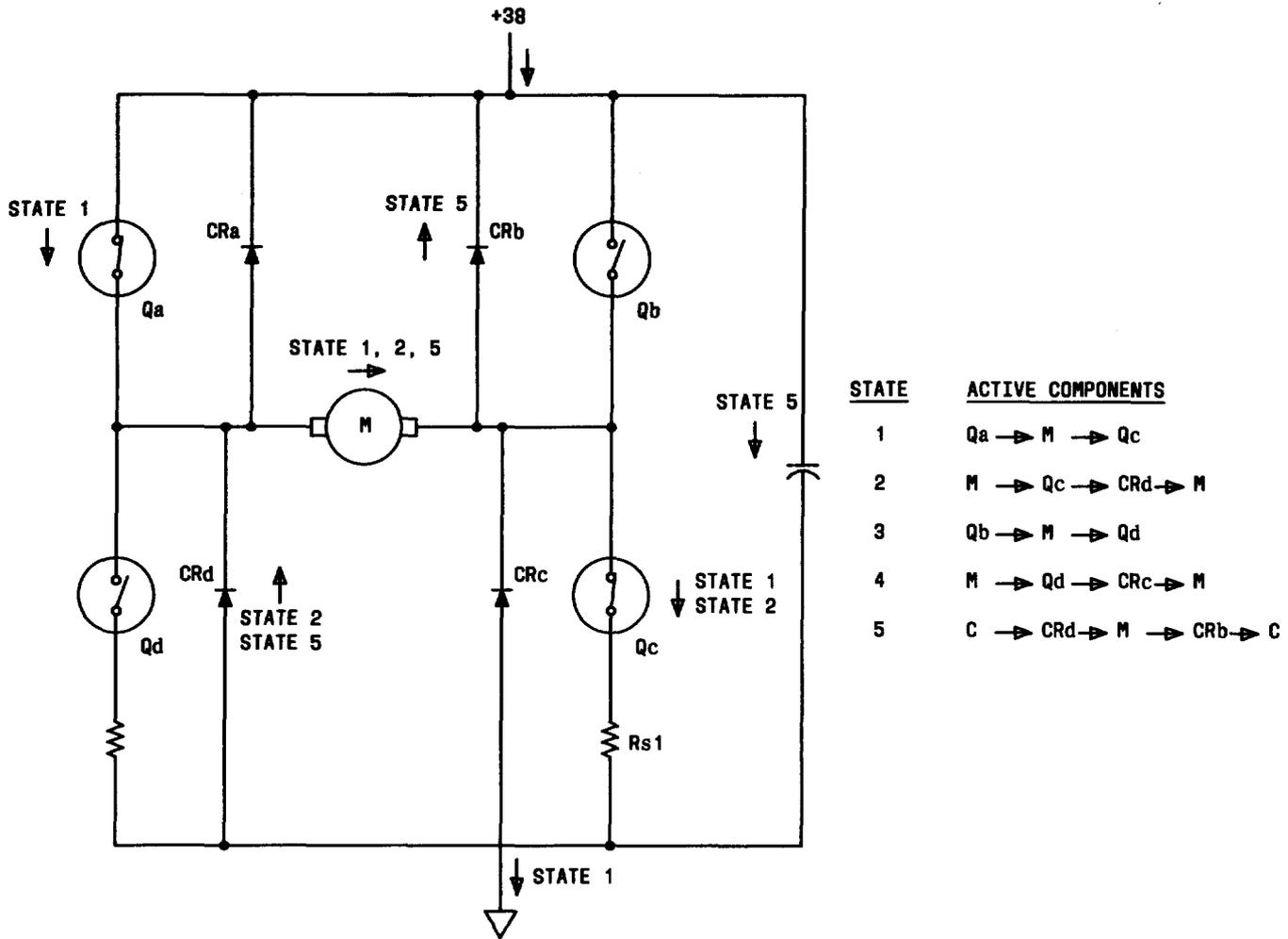
Fig. 12—Bridge Circuit
