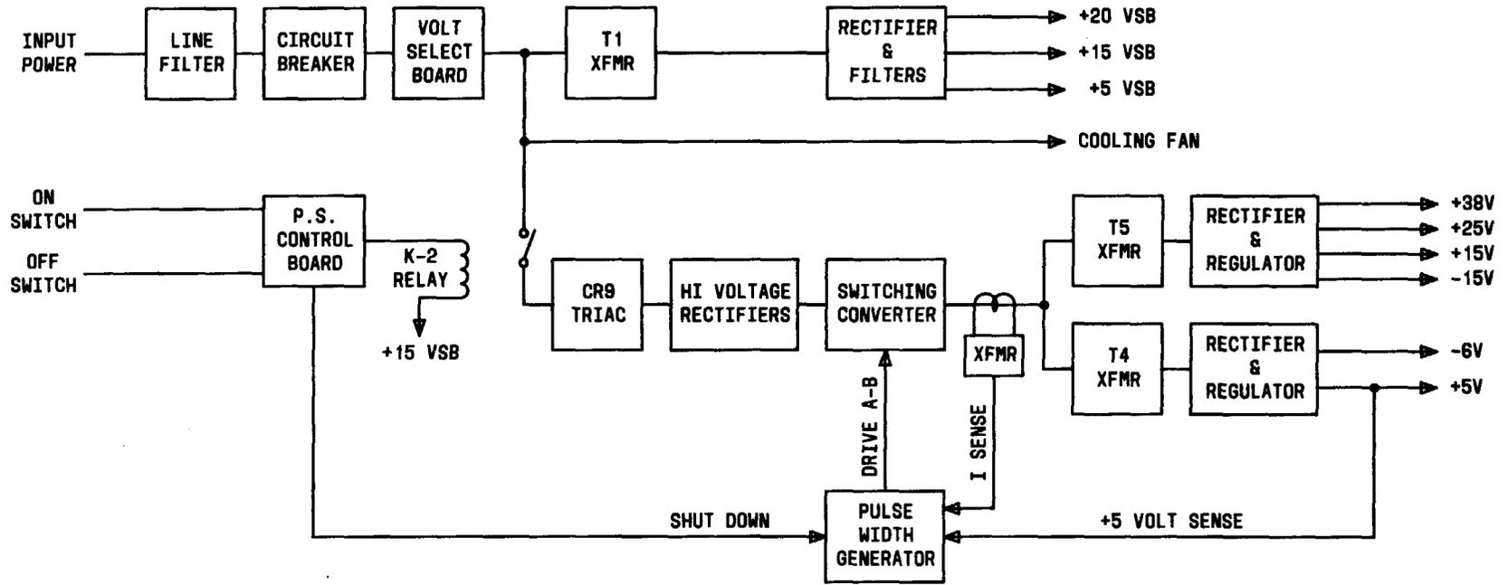
Fig. 10—Power Supply Block Diagram
