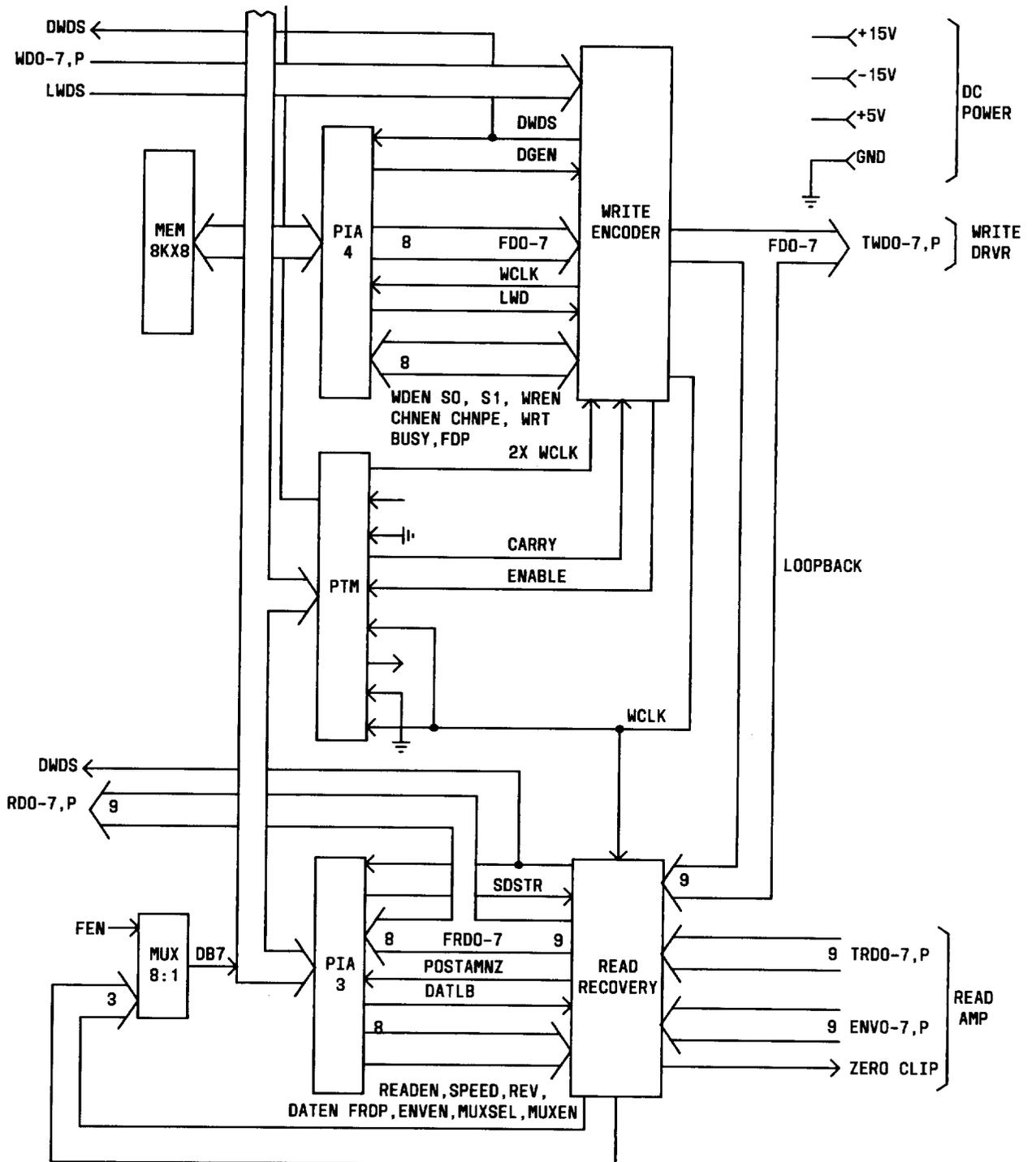
Fig. 8—Formatter/Control Block Diagram (Sheet 2 of 2)
