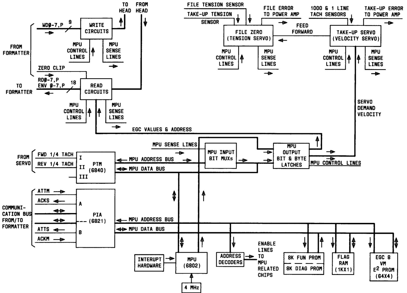
Fig. 9—Read/Write Servo Block Diagram
