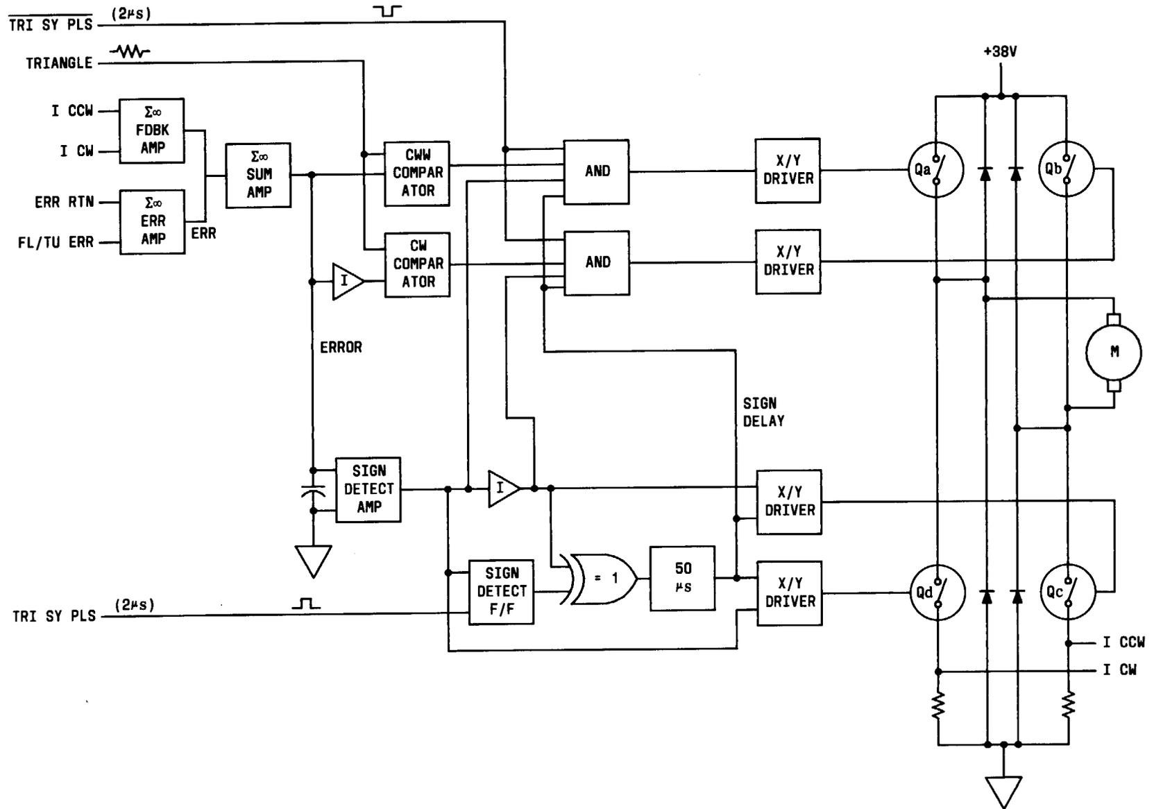
Fig. 11 — Power Amplifier Block Diagram
