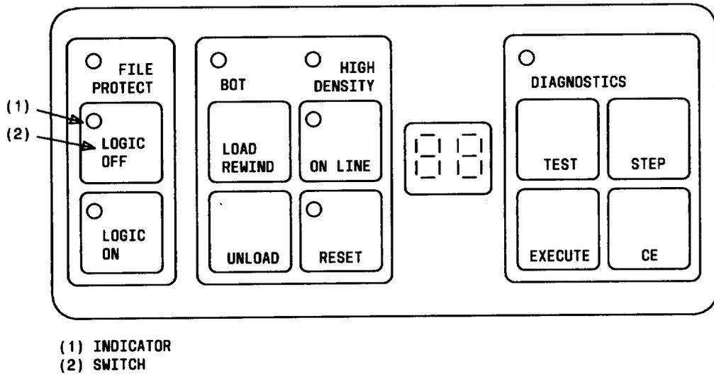
Fig. 4—Operator Control Panel
