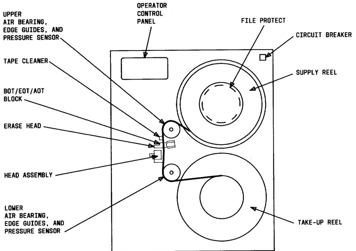
Fig. 5—Tape Deck (Front View)
