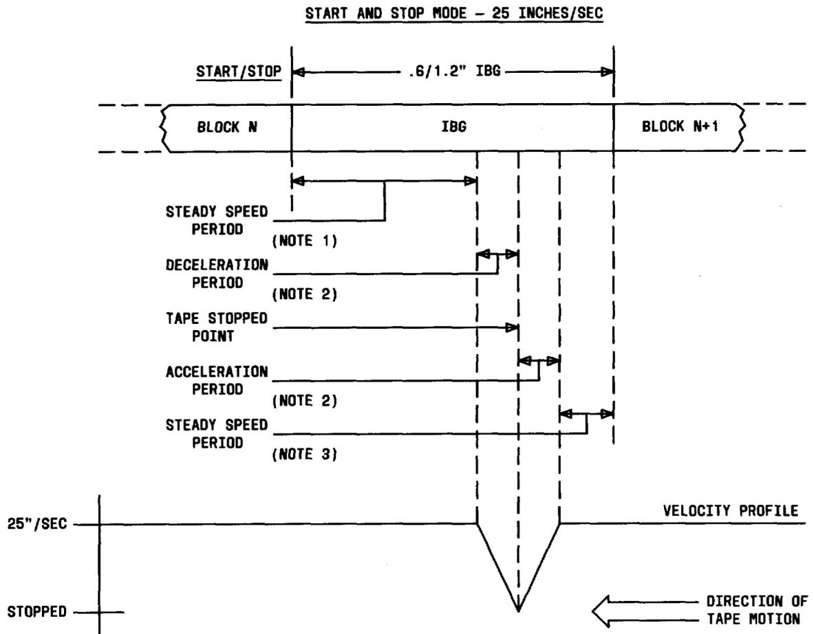
**Fig. 16—Start/Stop Mode Tape Motion Control**
