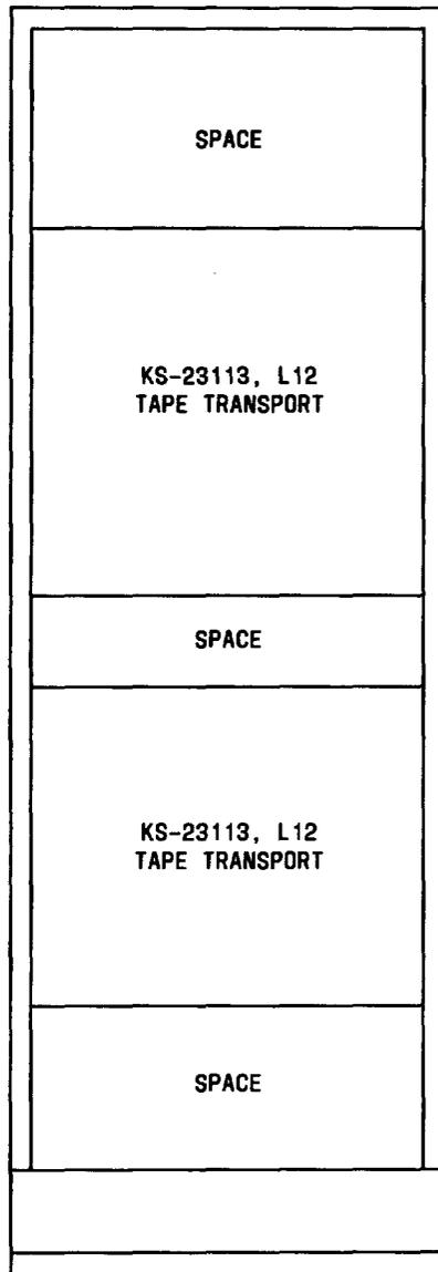
Fig. 2—Tape Transport Frame
