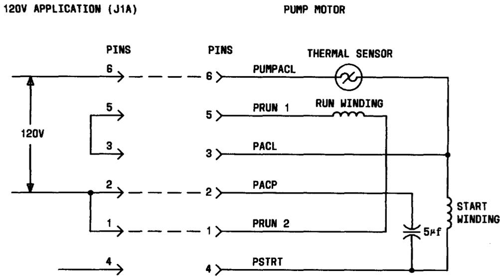
Fig. 14—Pump Motor Wiring Diagram
