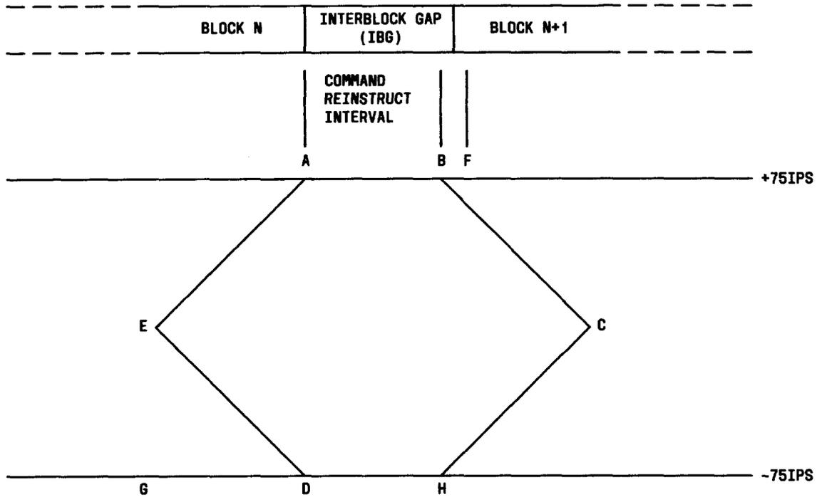
Fig. 17—Streaming Mode Velocity Diagram
