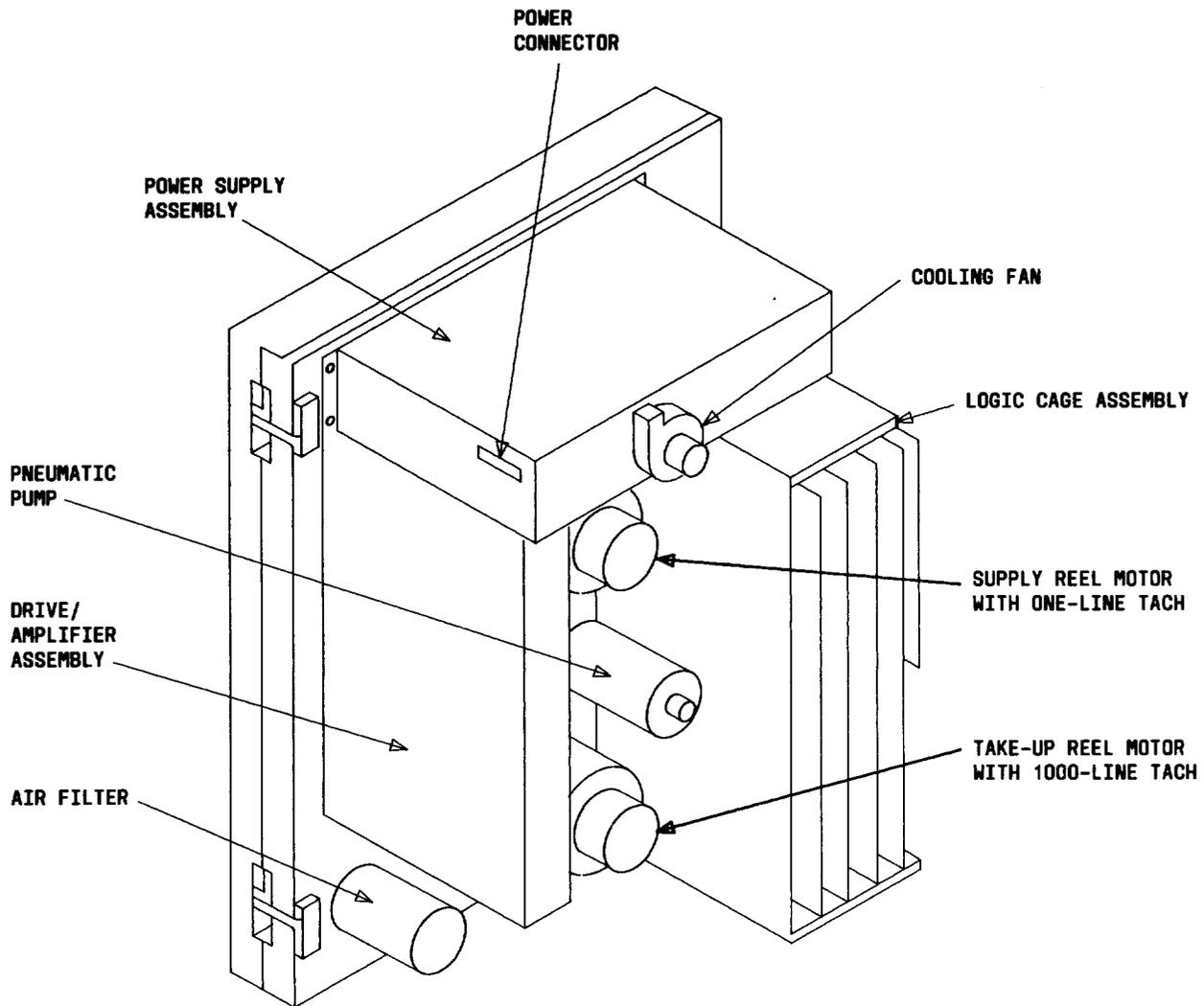
Fig. 6—Tape Deck (Rear View)
