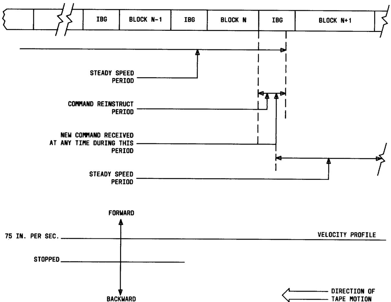
Fig. 18—Tape Motion Control (Nonstop)
