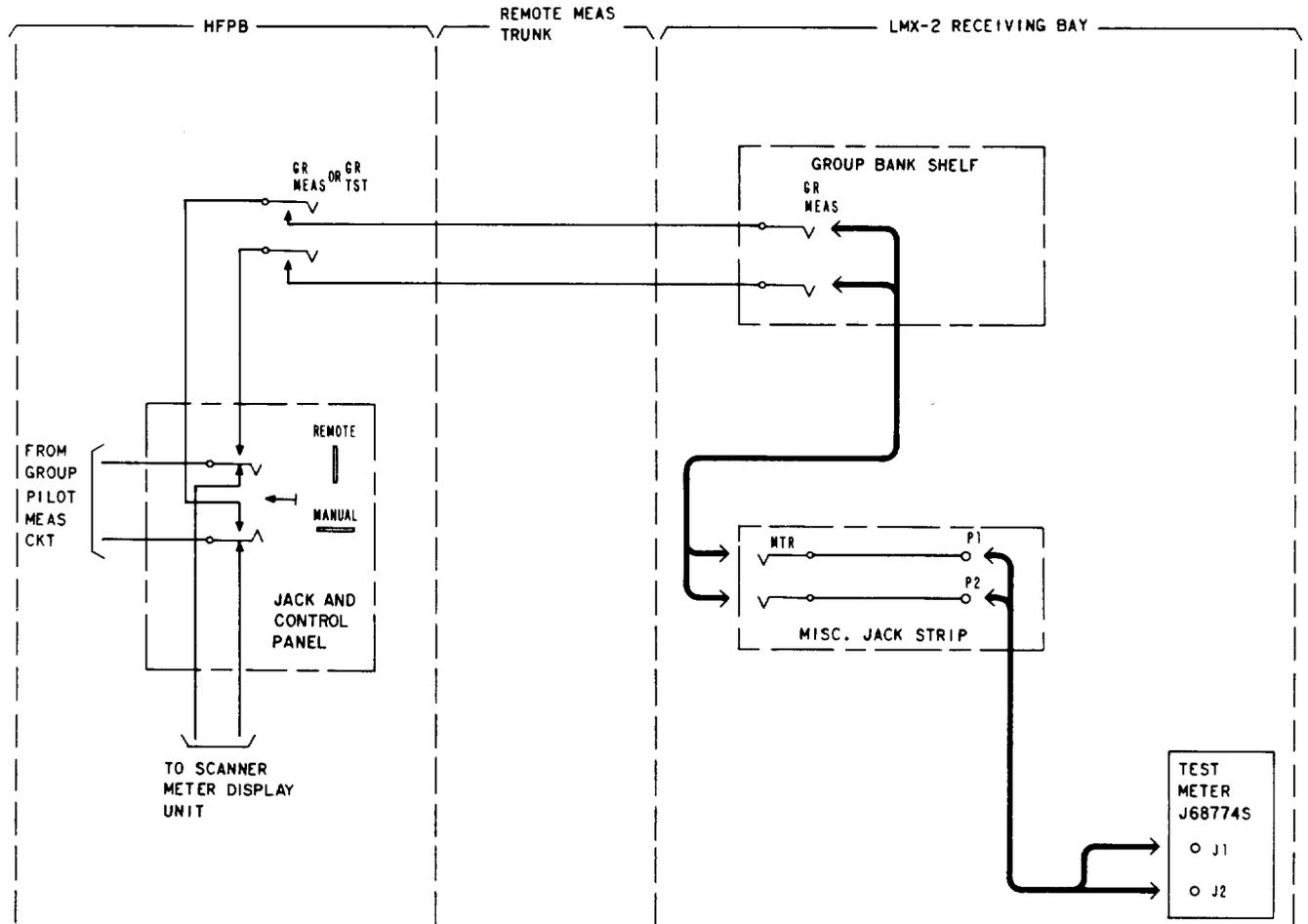
Fig. 9—Group Gain Remote Measuring Circuit
