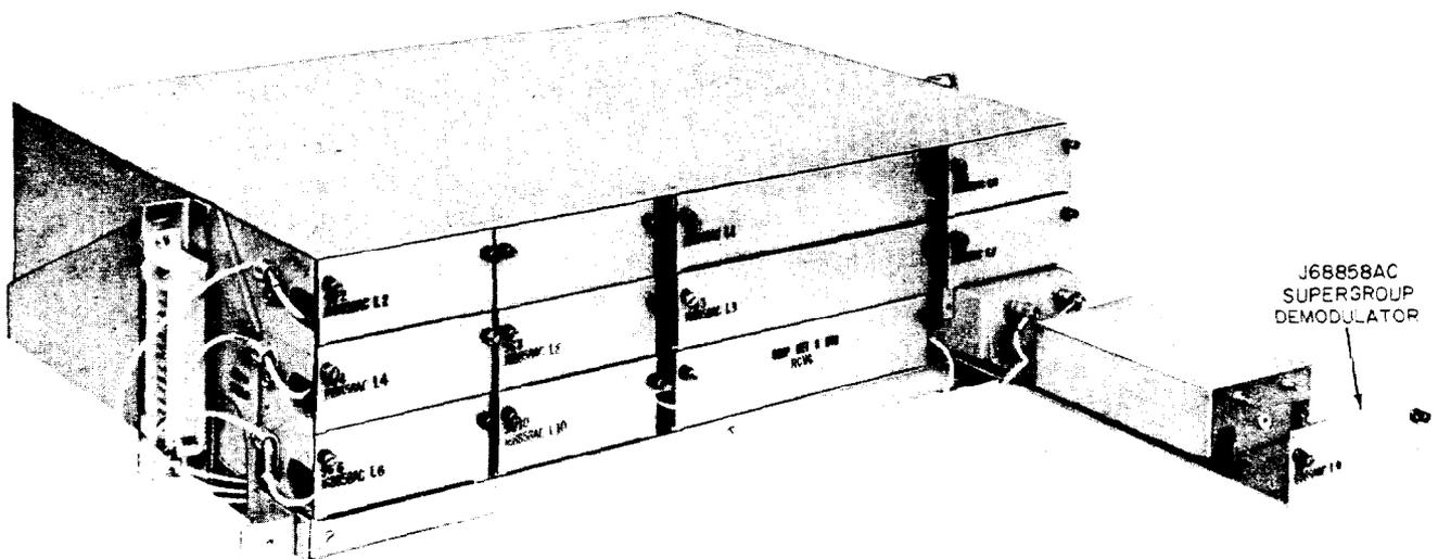
Fig. 2—C2A Supergroup Modulator Shelf Assembly J68858F
