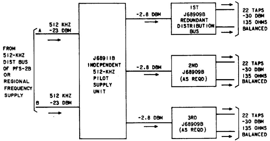
Fig. 2—Independent 512-kHz Pilot Supply and Distribution Circuit
