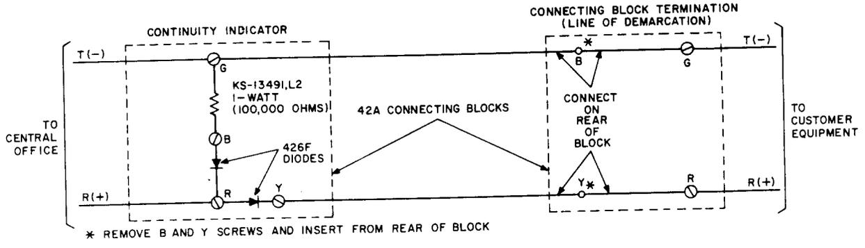
Fig. 24—DC Telegraph Loop Continuity Indicator—COAM Equipment, Neutral Operation
