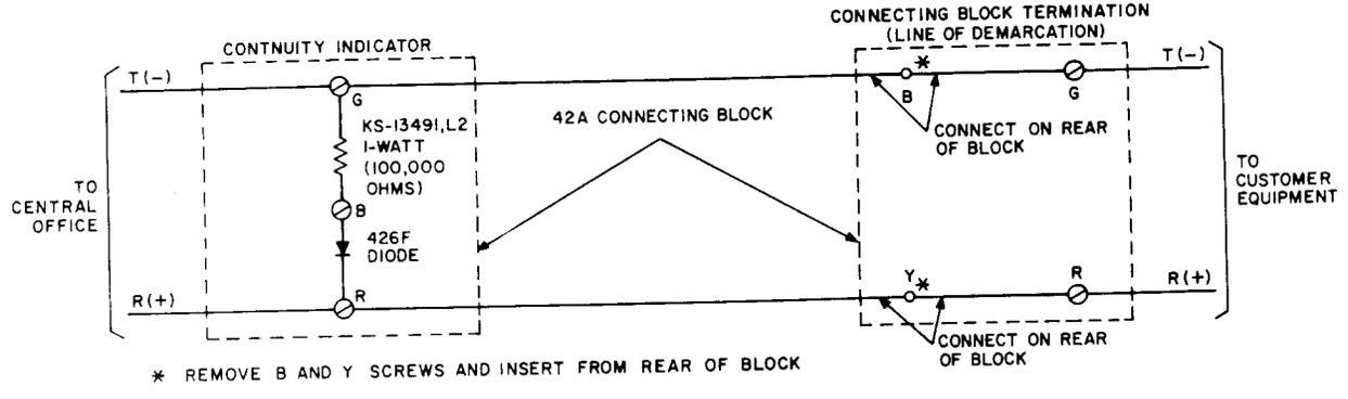
Fig. 25—DC Telegraph Loop Continuity Indicator—COAM Equipment, Polar Operation
