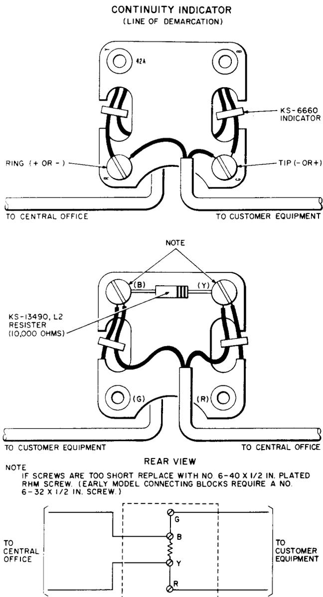
**Fig. 21—Radio Program Loop Continuity Indicator**
