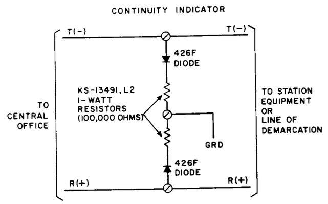
Fig. 26—DC Telegraph Loop Continuity Indicator (Alternate Method)
