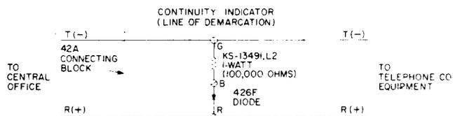
**Fig. 23—DC Telegraph Loop Continuity Indicator—TCM Equipment, Polar Operation**
