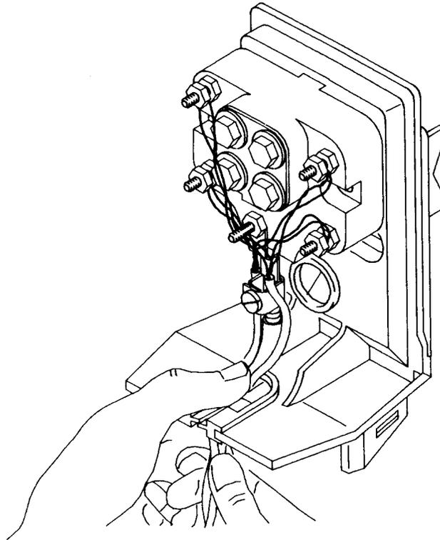
**Fig. 5—Placing Wires Through Horseshoe Grommet**
