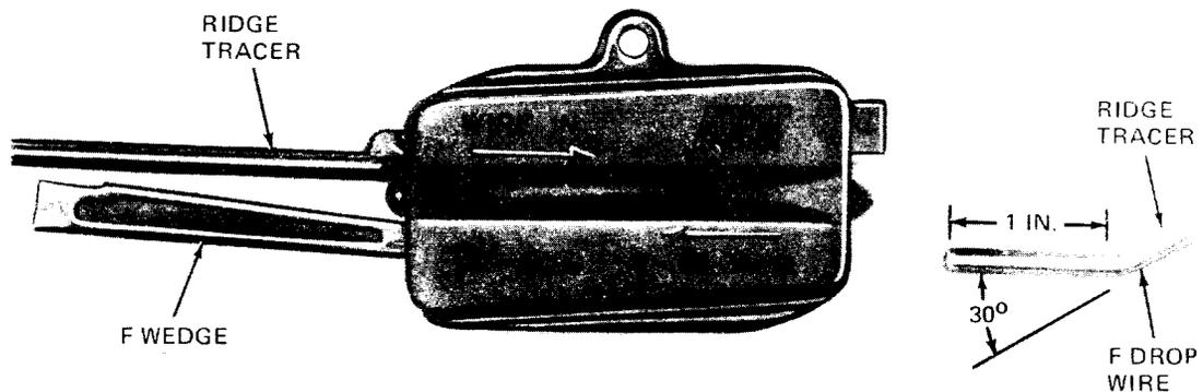
**Fig. 5—Aligning Ridge Tracers**
