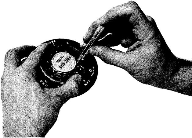
Fig. 4 — Removing Plastic Fingerwheel
