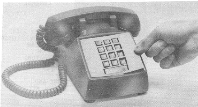
Fig. 3—Removing the Snap-In Faceplate
