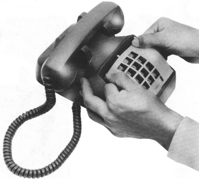
Fig. 4—Replacing the Snap-In Faceplate
