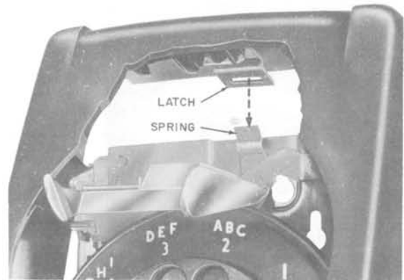
Fig. 4—Replacing Wall Telephone Set Housing
