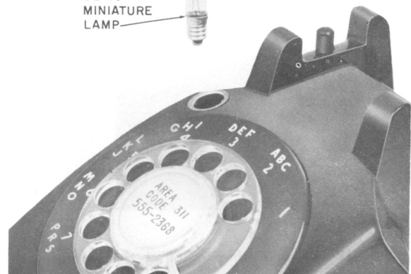
Fig. 15—Lamp Assembly, 500H/P Telephone Set
