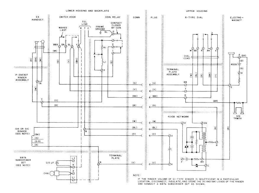
Fig. 1—236G Coin Telephone Set Connections
