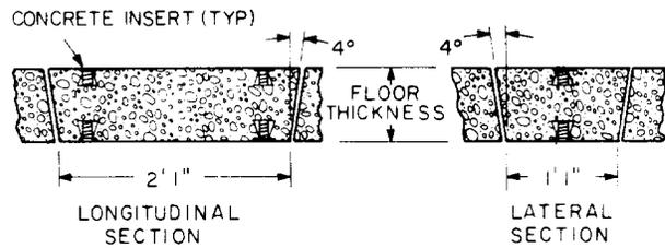
Fig. 11—Tapered Precast Concrete Cable Opening Plug-In Place
