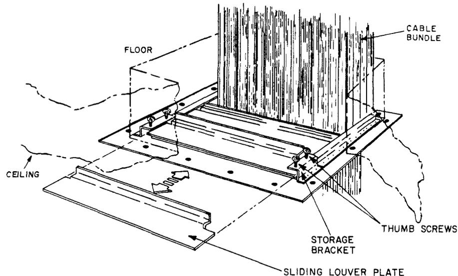
**Fig. 13—Adjustable Cable Hole Ceiling Plate for 12- by 24-Inch and 24- by 24-Inch Cable Openings**
