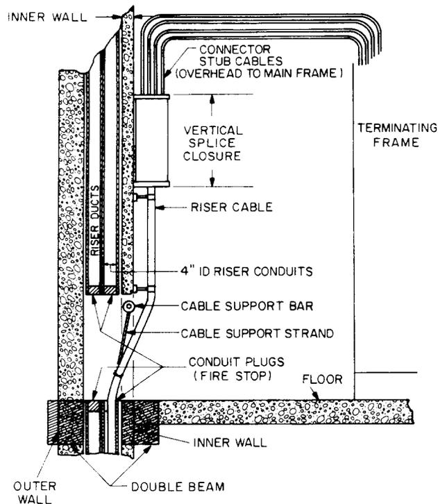
Fig. 4—Riser Cable System
