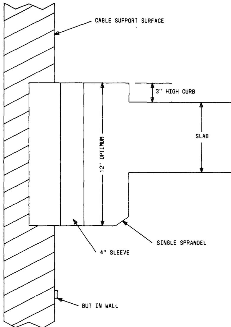
Fig. 1—Typically Upper Floor Riser Construction
