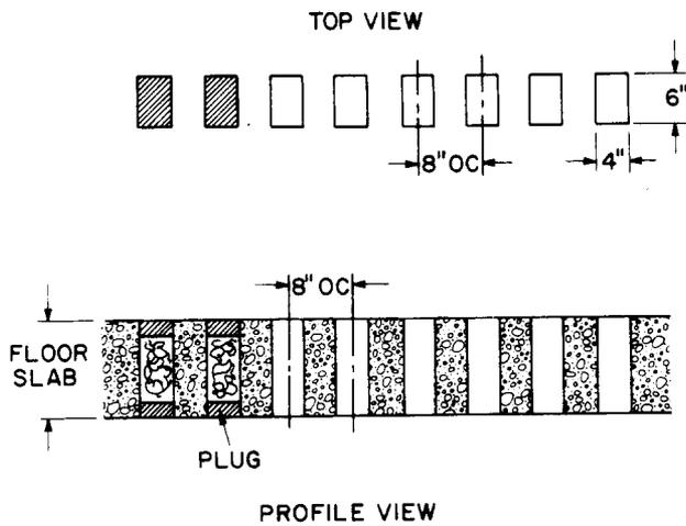
Fig. 5—Rectangular Frame Opening Pattern for the DSPF and LPCDF
