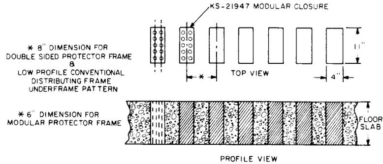
Fig. 7—Frame Opening Pattern for Modular Underframe Blocks
