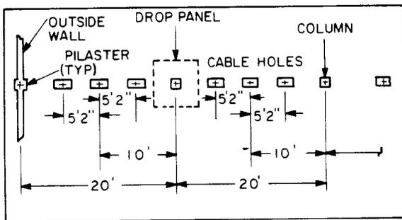
Fig. 10—Plan for Plugged Cable Openings for Future Use
