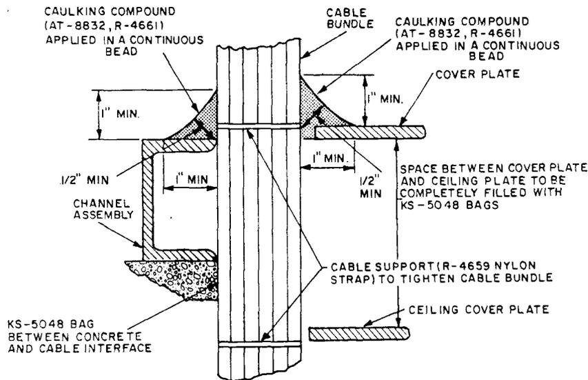
Fig. 14—Fire Stopping Arrangement for 12- by 24-Inch and 24- by 24-Inch Cable Openings
