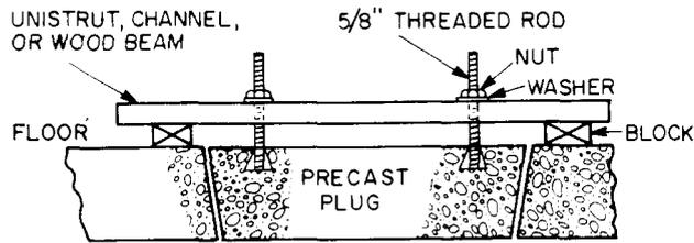
**Fig. 12—Removal of Precast Plug with Beam and Jack Screws**
