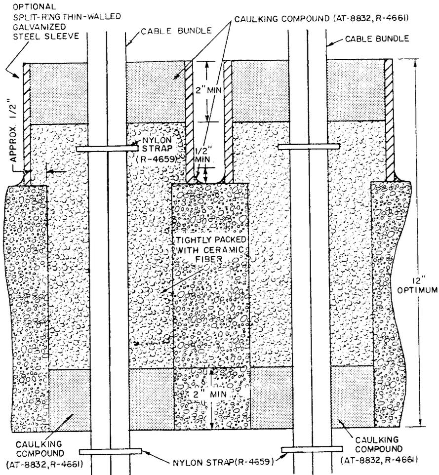
Fig. 9—Recommended Fire-Stopping Configuration for 2- by 6-Inch and 4- by 6-Inch Cable Holes
