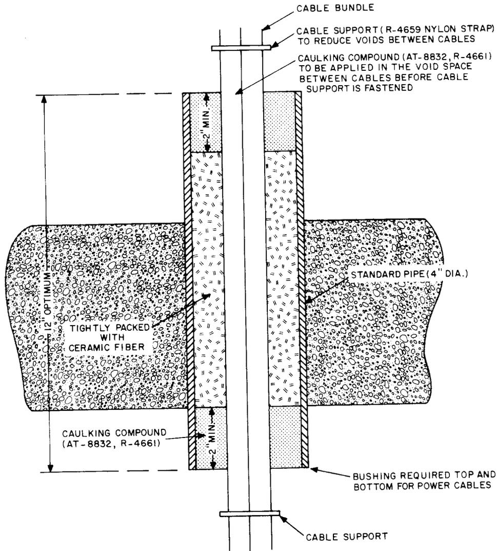
Fig. 3—Fire-Stopping Configuration for Circular Cable Openings
