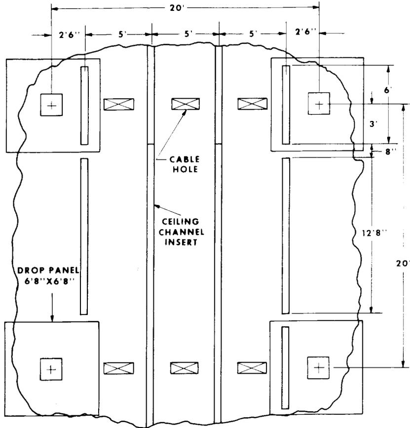
Fig. 5—Section of Equipment Room Showing Location of Channel Inserts (UNISTRUT) for Each 20' × 20' Bay
