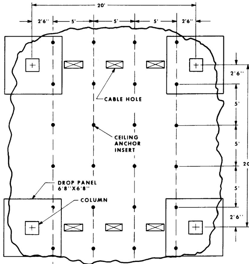
Fig. 4—Section of Equipment Room, Showing Location of Anchors
