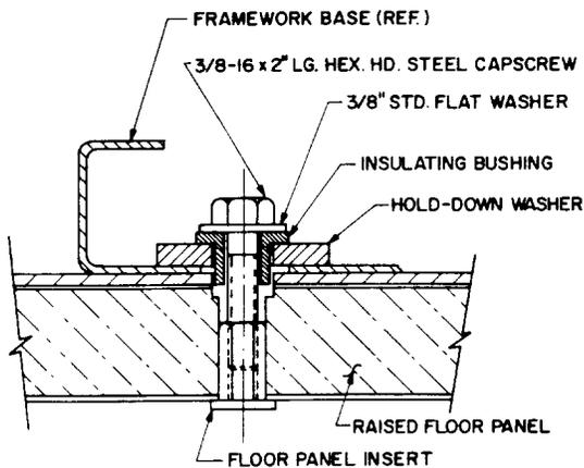
Fig. 7—Typical Frame Hold-Down for Installation on Wood-Core Floor Panels
