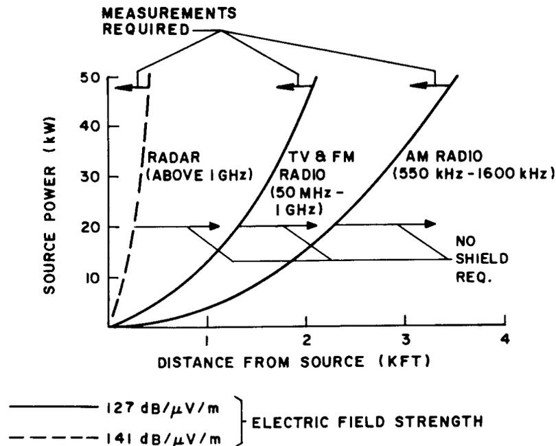
Fig. 2—Relationship of RFI Source Power and Distance to Maximum Permissible Field Strengths For ESS Equipment
