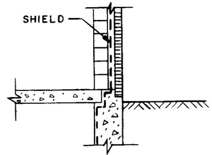
(1) BRICK-AND-BLOCK WALL AT FOUNDATION
