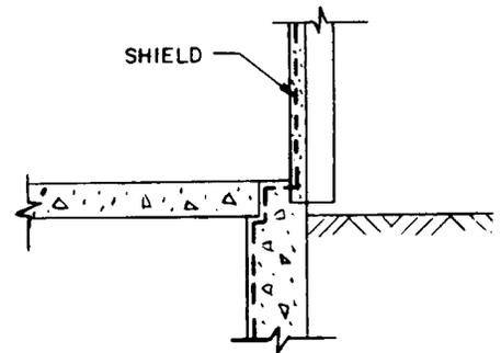
(2) PRECAST CONCRETE WALL AT FOUNDATION
