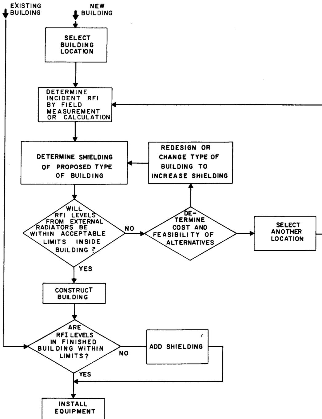
Fig. 1—Basic Procedure For Minimizing Potential RFI Problems
