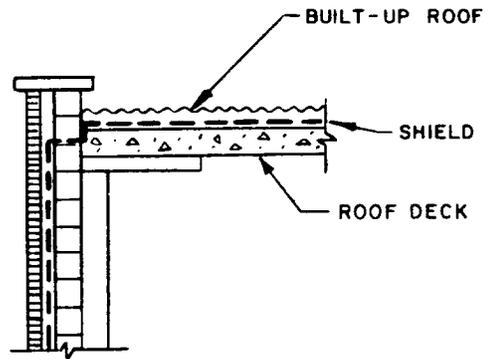
(1) REINFORCED CONCRETE FRAME WITH BRICK-AND-BLOCK CAVITY EXTERIOR WALL
