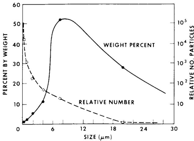
Fig. 3—Plot of Representative Particle Distribution in Atmosphere. Particles Below 2 Micrometers in Size Account for Small Percentage of Weight of Total Particles but Over 99% of Total Number. Such Fine Dusts are Responsible for Most Equipment Soiling.
