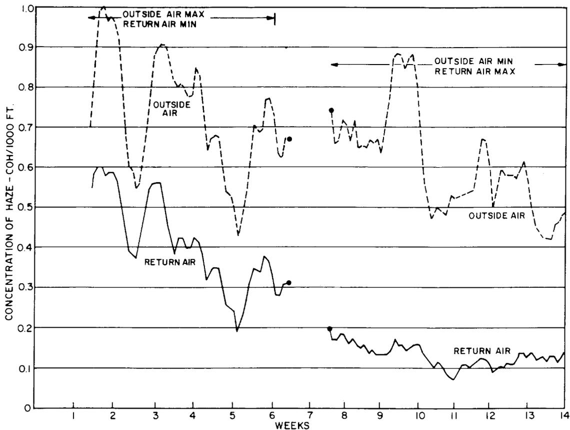
Fig. 11—Category C—Central Office Air Sampling Concentration of Haze/1000 Ft vs Time for 7-Day Moving Average
