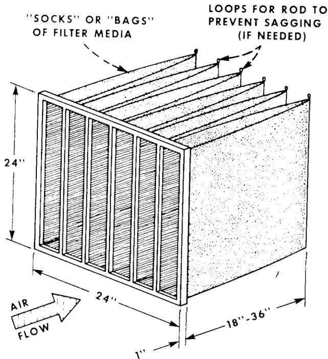
**Fig. 8—High-Efficiency Filter for Removal of Fine Dust (Nonsupported Type III)**
