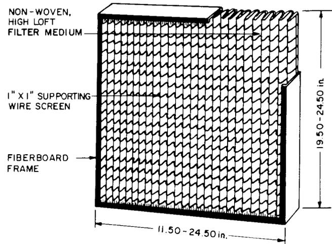
**Fig. 6—Internally Supported Filter with Pleated Cotton Media**
