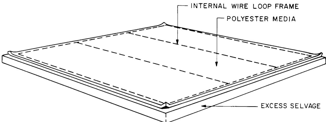
Fig. 5—Internally Supported Filter
