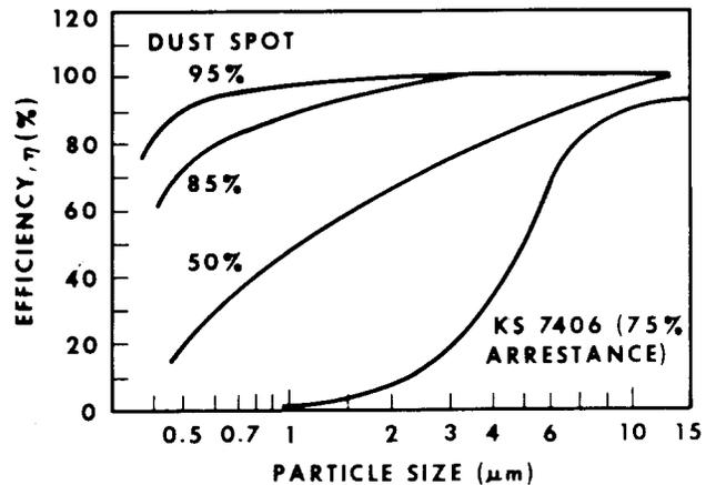
Fig. 4—Plot of Filter Efficiency vs Particle Size for High and Low Efficiency Filters
