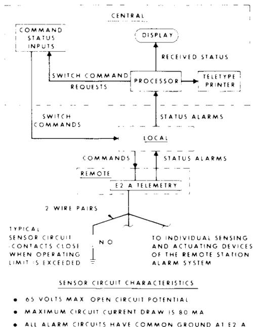
Fig. 2—Telemetry Alarm System Block Diagram
