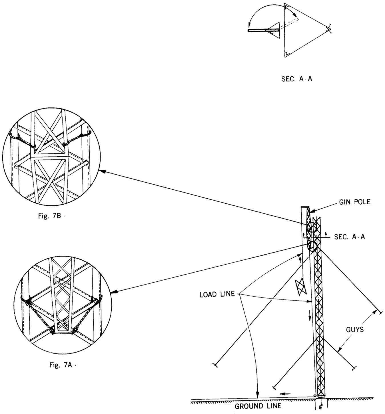
Fig. 7 - Typical Gin Pole Set-up for Hoisting Tower Sections
