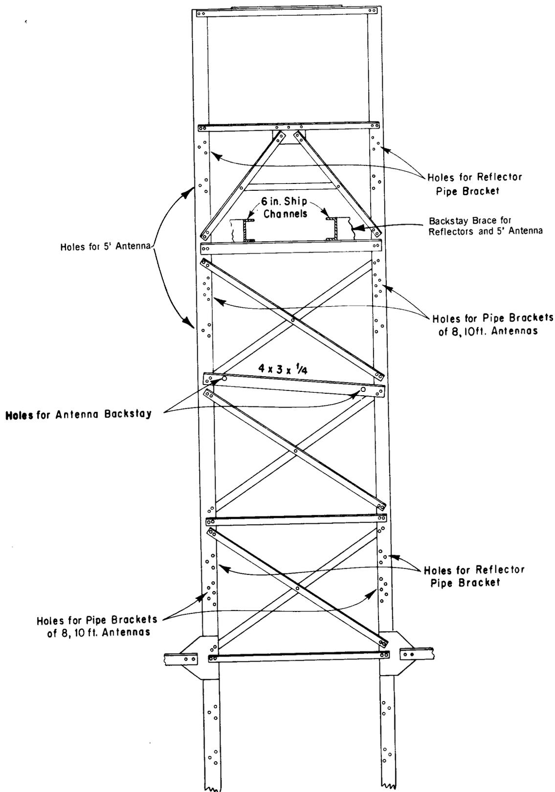
Fig. 12 - Locations for Antenna and Reflector Pipe Brackets
