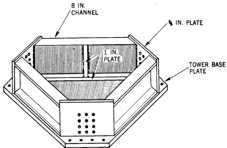
INTERNAL BRACING OF TOWER BASE
