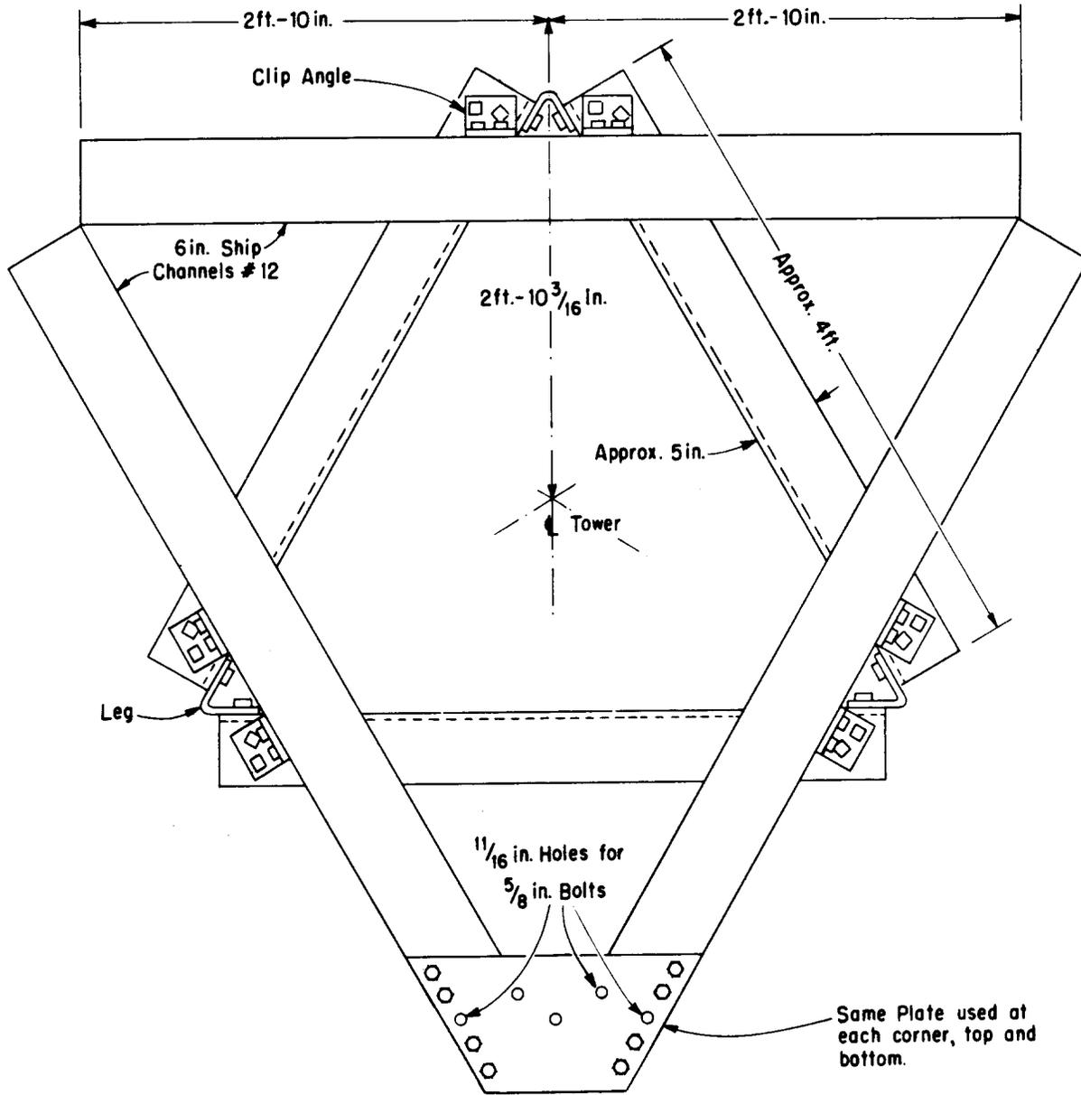
Fig. 11 - Triangular Brace for Attachment of Reflector Backstays
