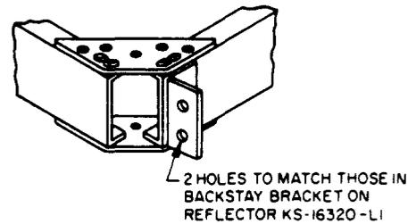
FIG 3C - REFLECTOR BACKSTAY MOUNT
