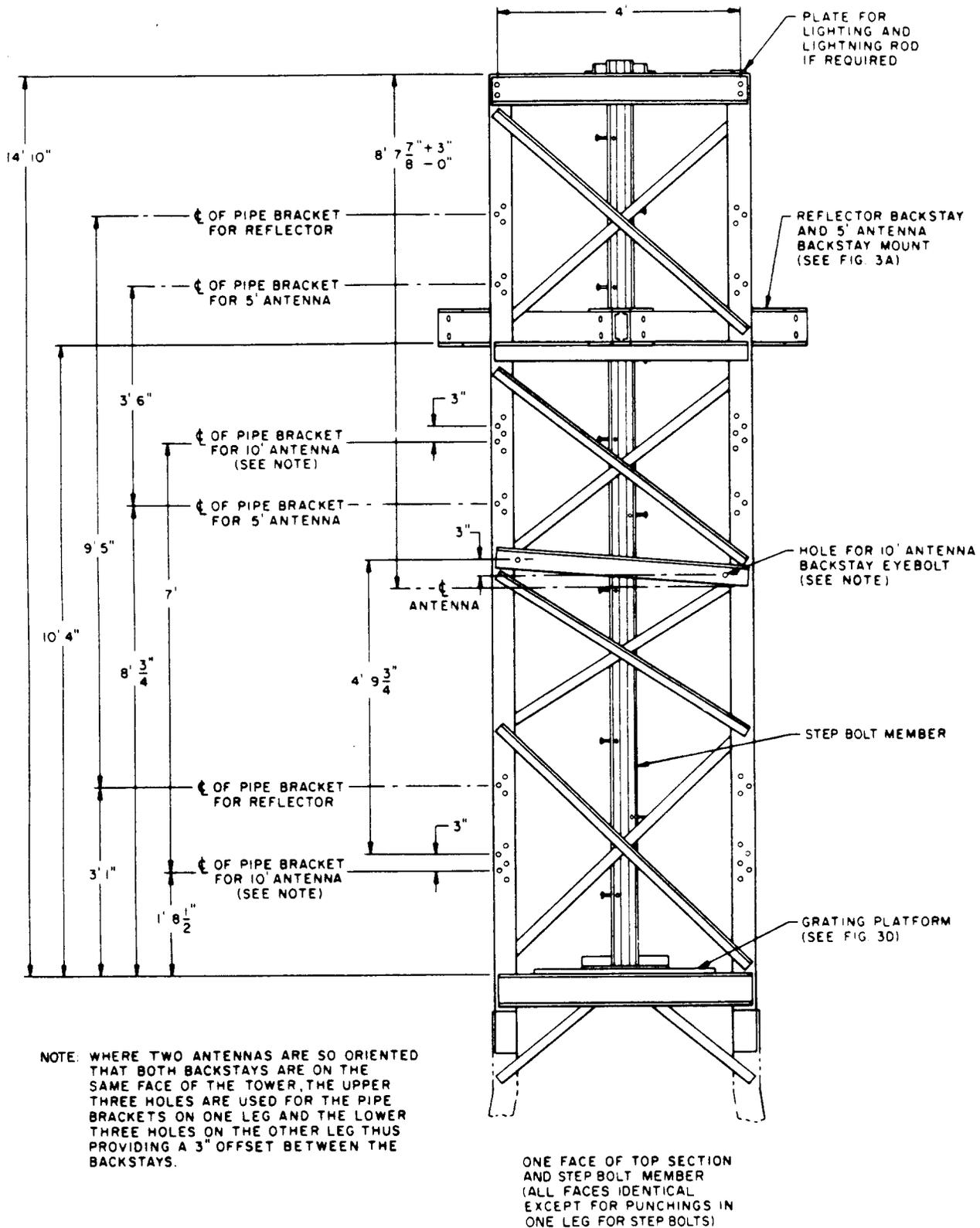
Fig. 2 - Top Section of C Self-Supporting Tower
