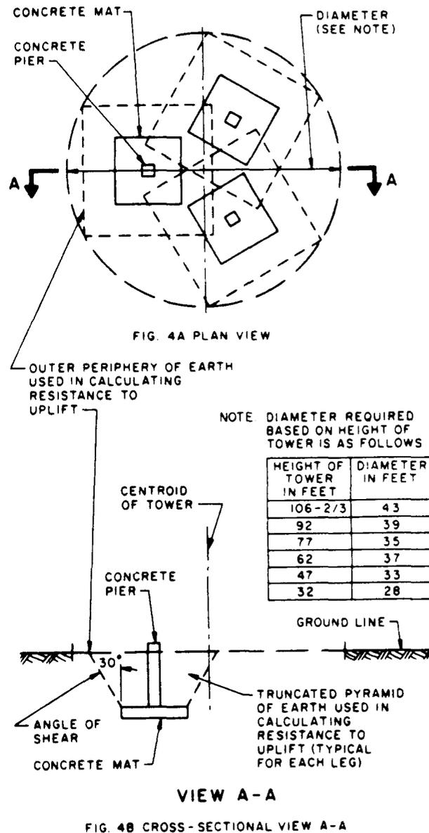
**Fig. 4 - Land Area Required for Tower Foundation**
