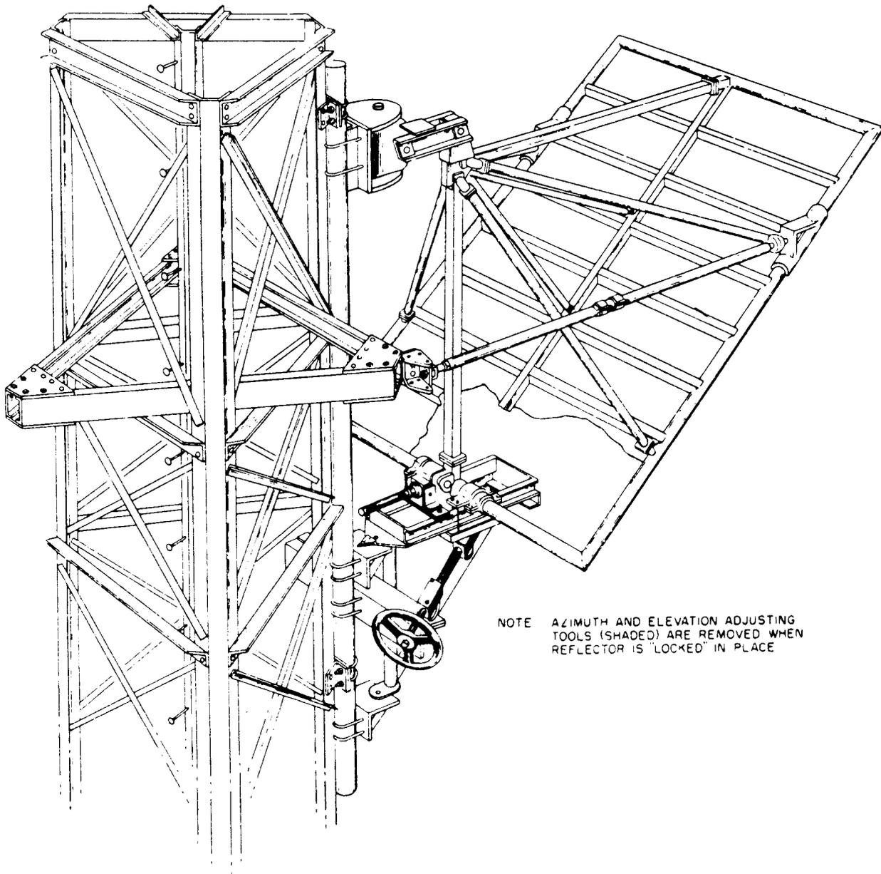
NOTE AZIMUTH AND ELEVATION ADJUSTING TOOLS (SHADED) ARE REMOVED WHEN REFLECTOR IS "LOCKED" IN PLACE
