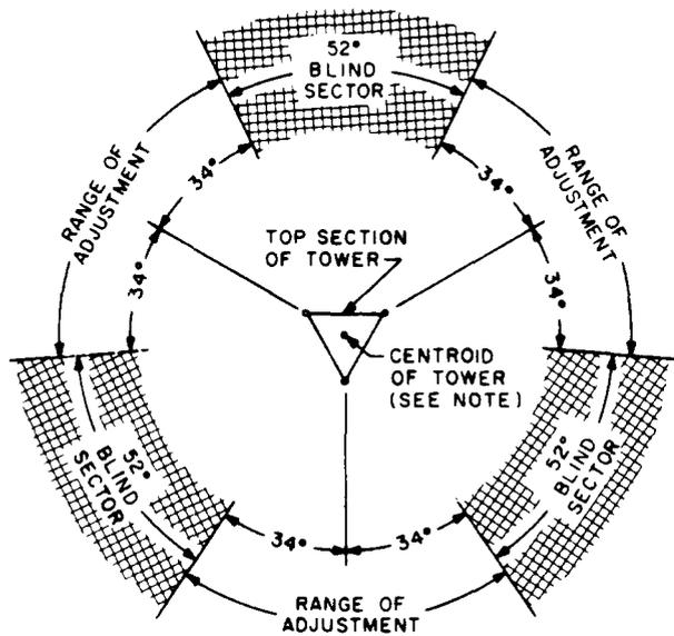
FIG. 8A AZIMUTH LIMITATIONS OF KS-15852
