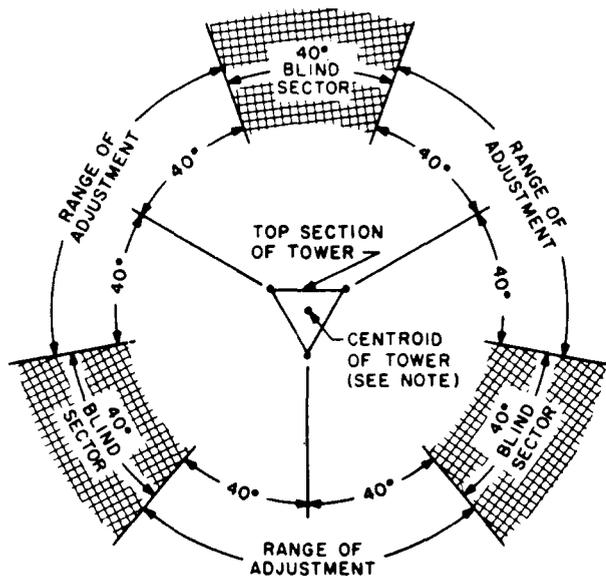
FIG. 8B AZIMUTH LIMITATIONS OF KS-16320-LI
