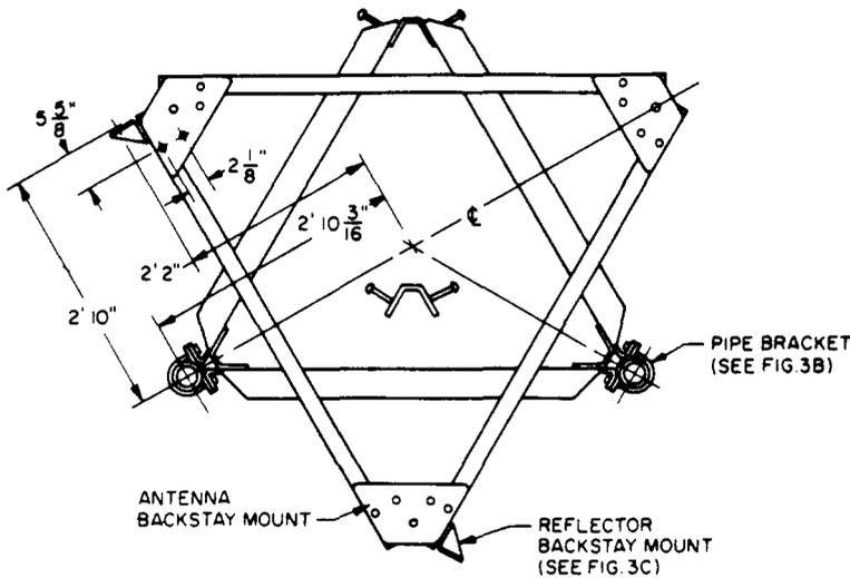
FIG 3A - REFLECTOR BACKSTAY AND 5' ANTENNA BACKSTAY MOUNT
