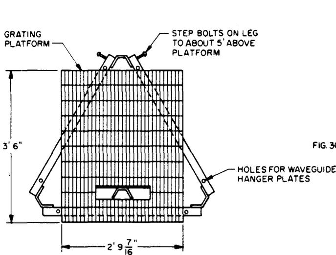
FIG 3D - GRATING PLATFORM AND STEP BOLT MEMBER BASE
