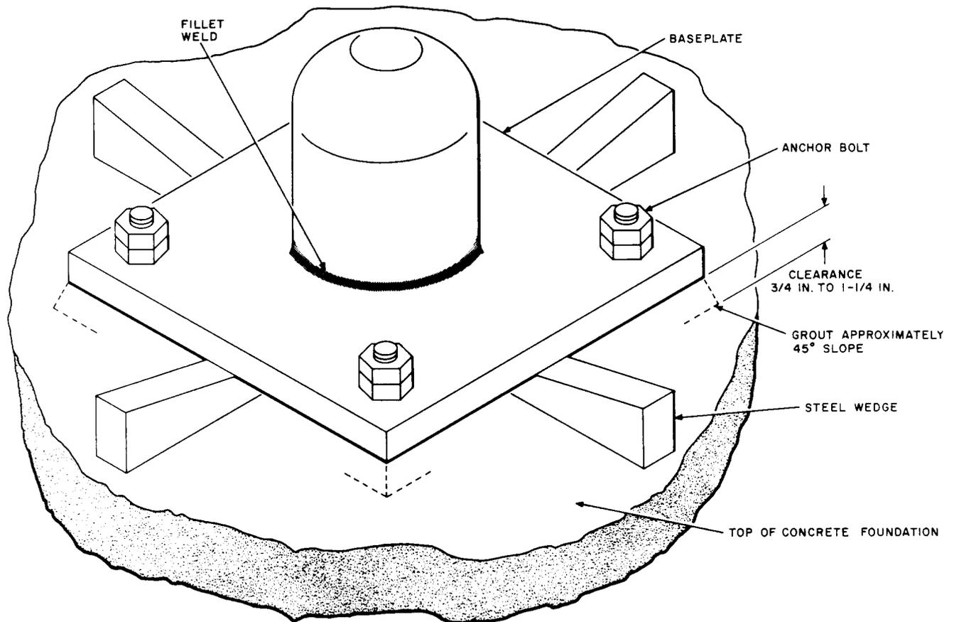
Fig. 1—Installation of Base Plate Assembly
