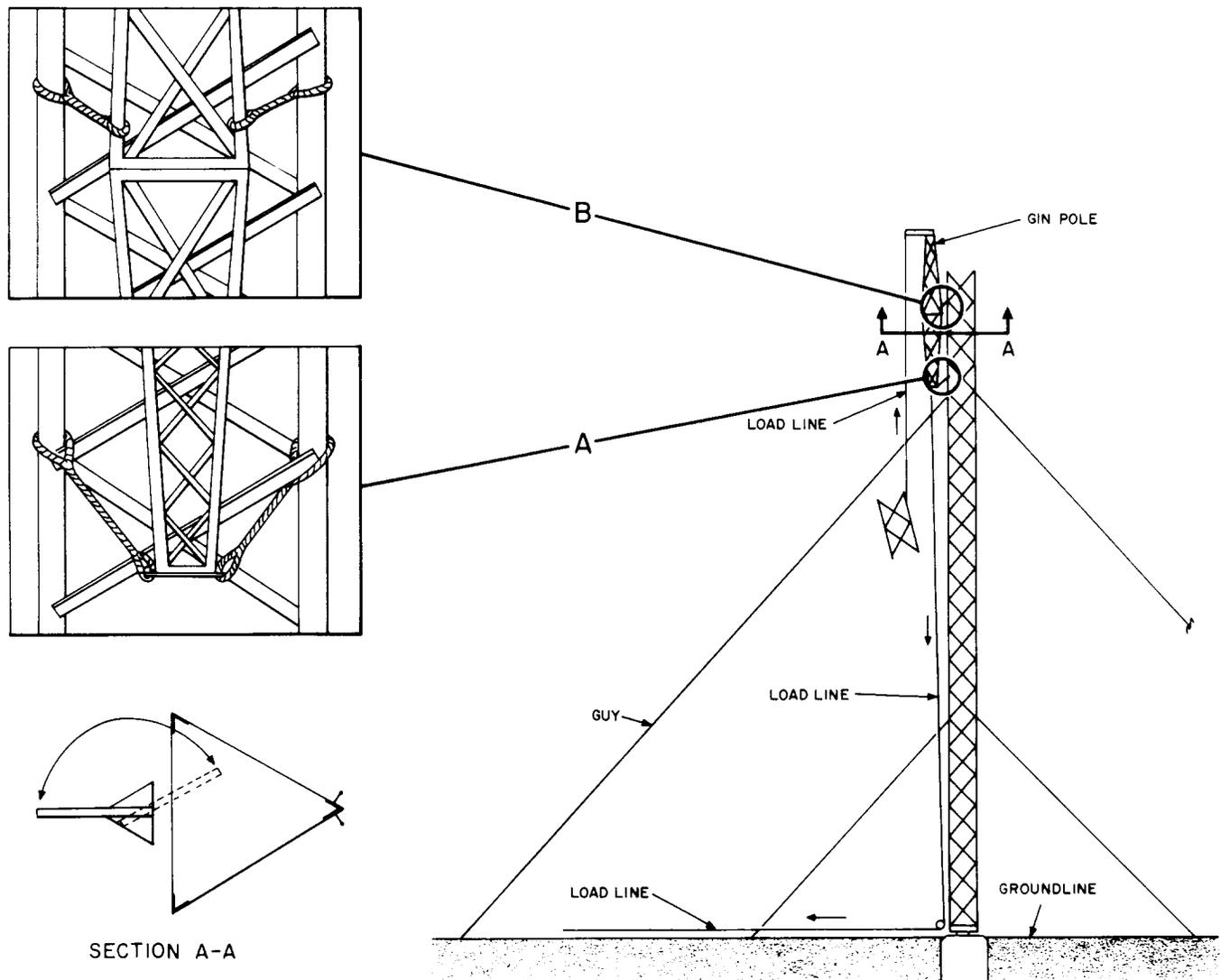
Fig. 5—Typical Gin Pole Setup for Hoisting Tower Sections
