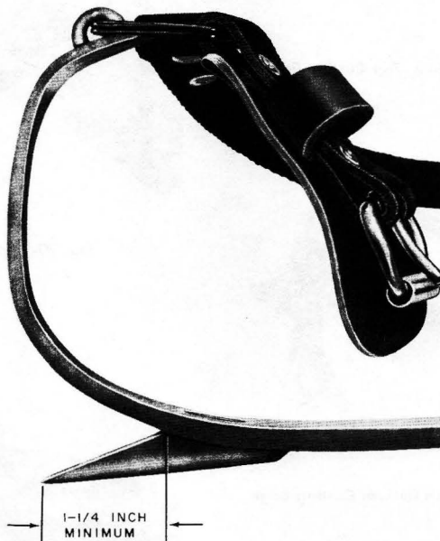
Fig. 22—Gaff Sharpened to Minimum Length
