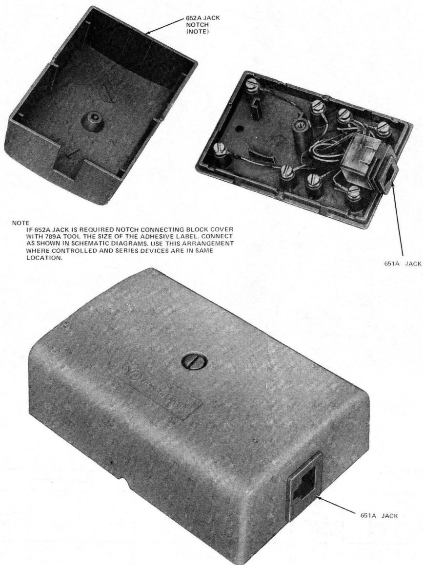
Fig. 14—635B Connecting Block
