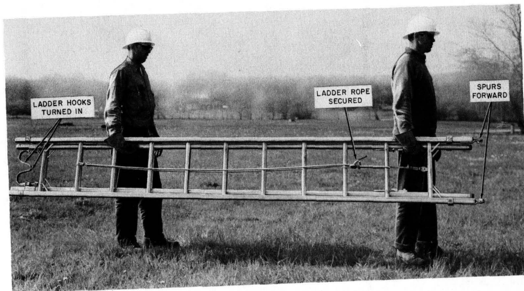
Fig. 7—Two-Person Method of Carrying an Extension Ladder
