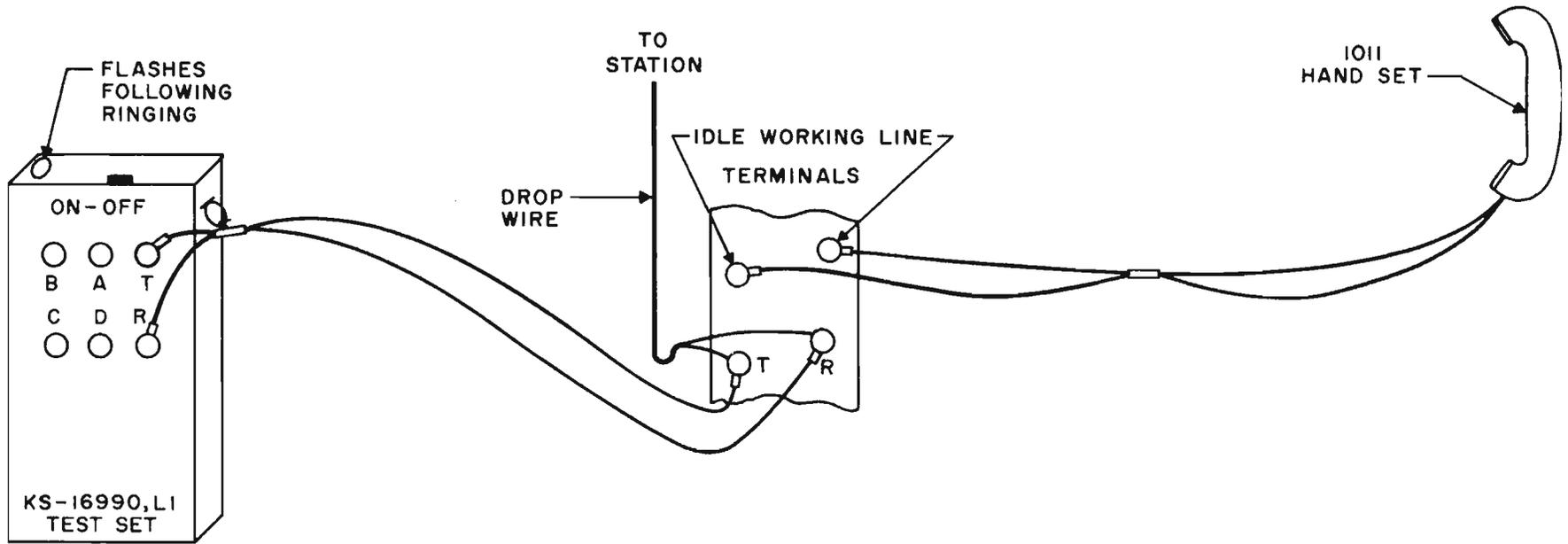
1. Slide ON-OFF switch to OFF position.
