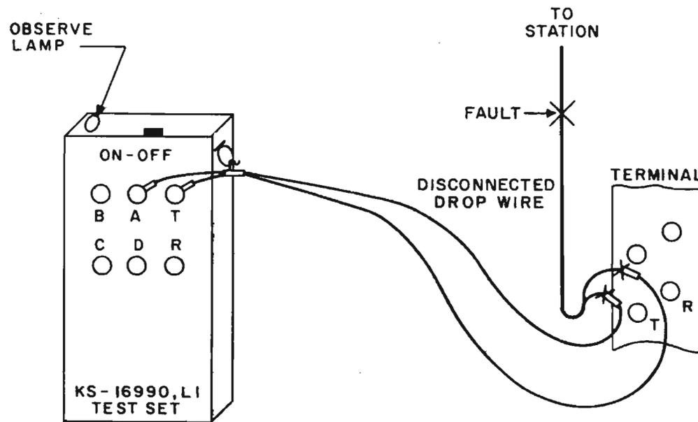
1. Place banana plugs of test cord into jacks A and T of test set.
