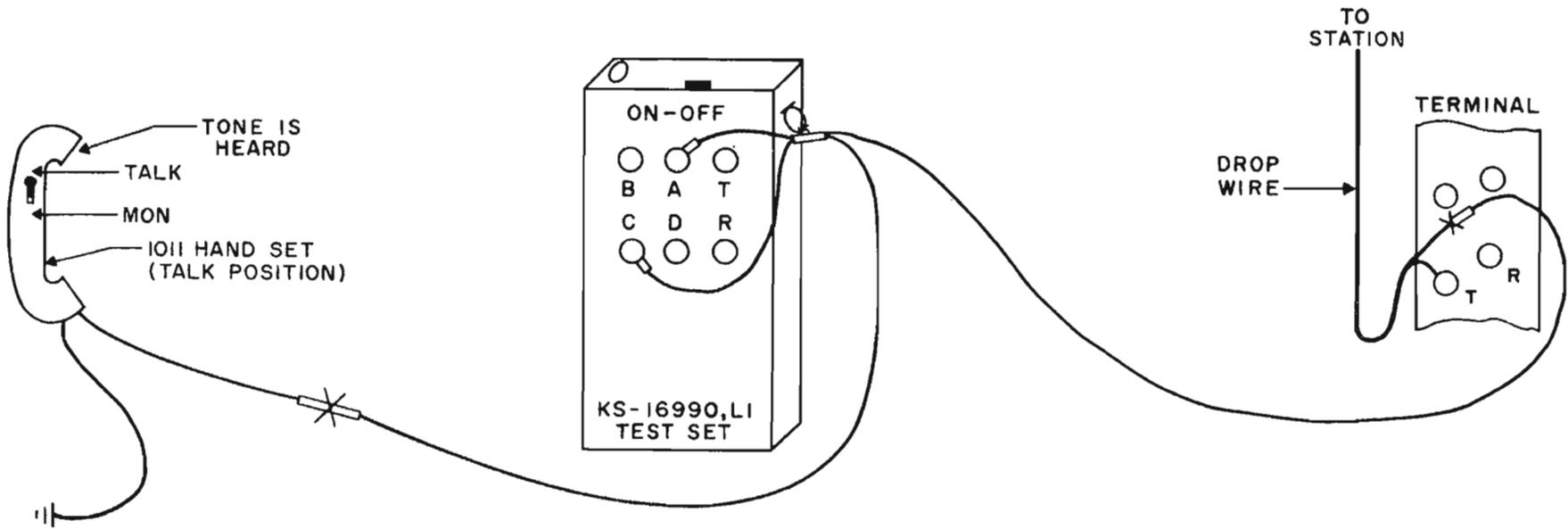
1. Identify Tip and Ring of line as described in Fig. 4 of this section.
