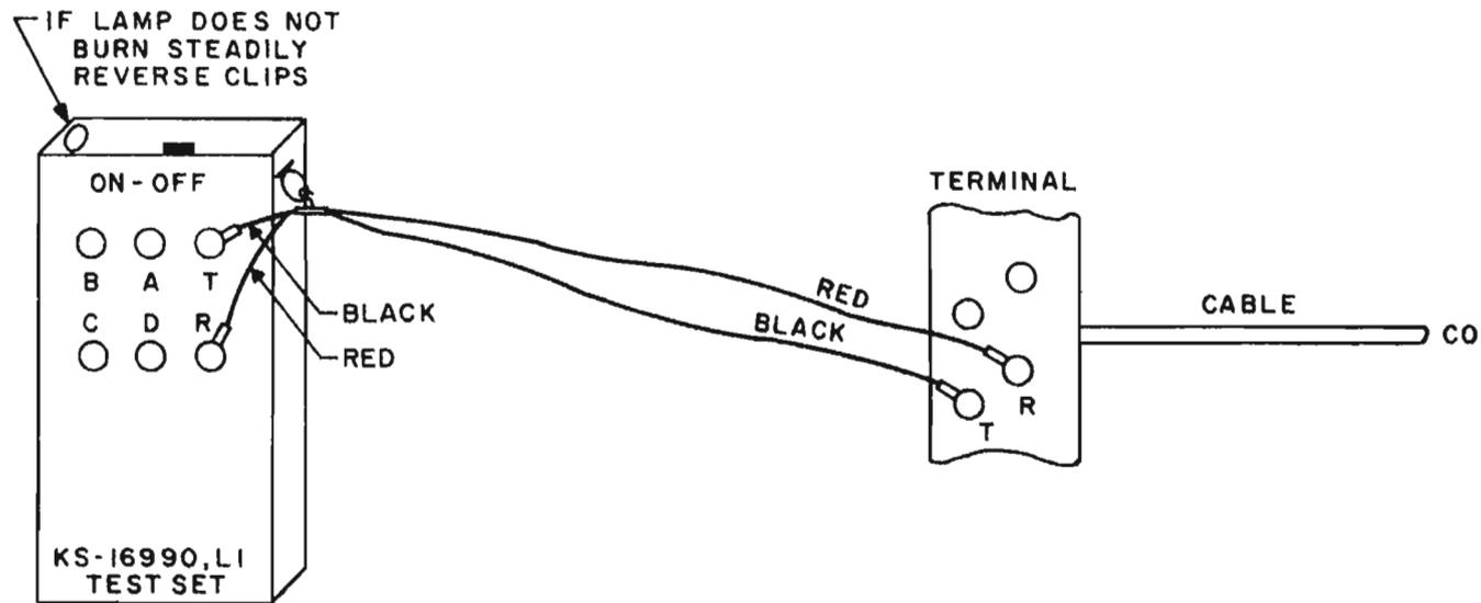
1. Place banana plugs of test cord in jacks *T* and *R* of test set.
