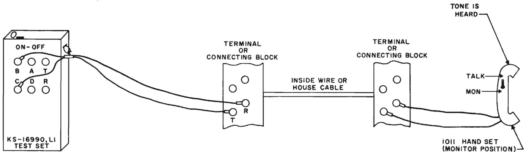
1. Place banana plugs of test cord in jacks *B* and *C* of test set.
